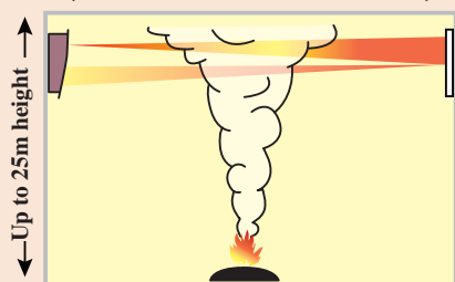
operation of reflective type optical beam smoke detector
