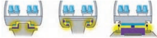
Electromagnets on the guideway levitate the car. Electromagnets on the cars lift the cars. Permanent magnets levitate over passive coils.
