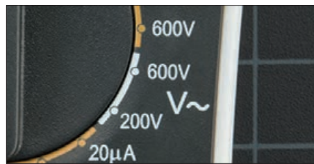
Use the V with a wavy line to measure AC Voltage
