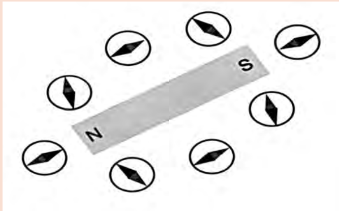
The compass shows how the magnetic force surrounds a magnet
