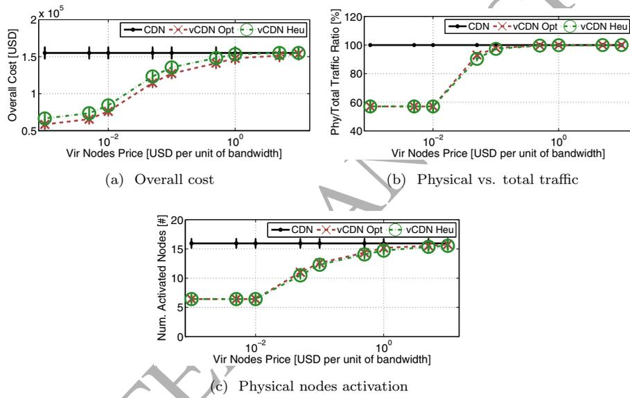
Figure 4: *Effect of the vCDN Price.* Plots 4a-4c show the effect of the virtual nodes pricing on the overall cost (Fig. 4a), the fraction of traffic served by the physical infrastructure (Fig. 4b) and the number of physical nodes activated (Fig. 4c), for different solution algorithms as well as a physical-only infrastructure (denoted in the figures with CDN).
