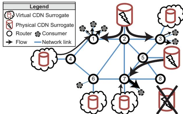
Figure 1: *System model*. The network is composed by consumers, routers, virtual and physical CDN surrogates. Our proposed optimization model selects (1) the planning of physical CDNs and (2) request routing.
