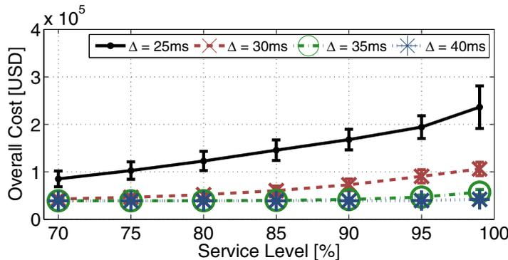
Figure 2: *Effect of the Service Level and Delay.* The figure shows the overall cost as a function of the desired service level ( $\epsilon$ ) and for different delays ( $\Delta = \{25, 30, 35, 40\}$  ms).
