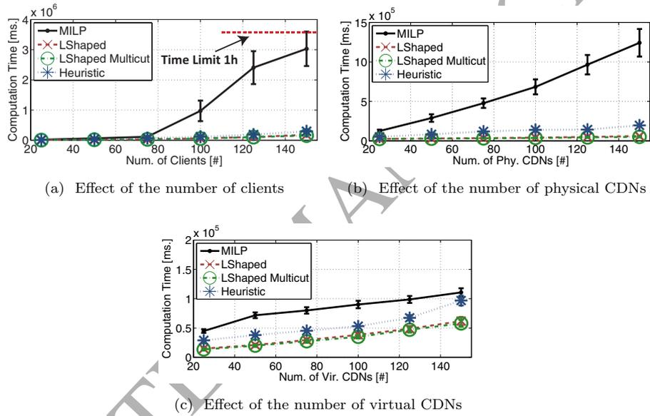
Figure 5: *Execution time*. Plots 5a-5c show the behavior of the different solution algorithms as a function of the number of clients as well as the number of surrogate nodes. We observe that the number of clients has the most remarkable effect on the execution time.
