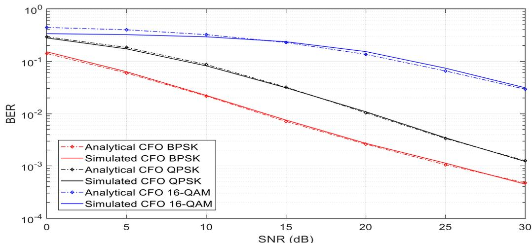
Fig. 6 Analytical BER Vs Simulated BER.
