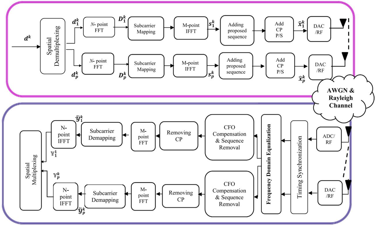
Fig. 3 Block Diagram of MIMO-Single-carrier FDMA system.
