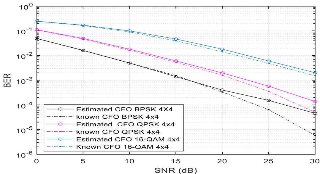
Fig. 10 Estimated CFO Vs Known CFO through proposed MIMO-SC-FDMA 4 x 4 system.
