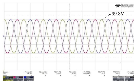
Fig. 17. Phase back EMF at the base speed 214rpm (experimental)
