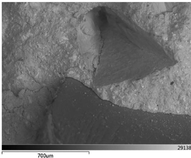
Fig. 6. SEM image of PET3 showing debonding of plastic particle on split cylinder surface.
