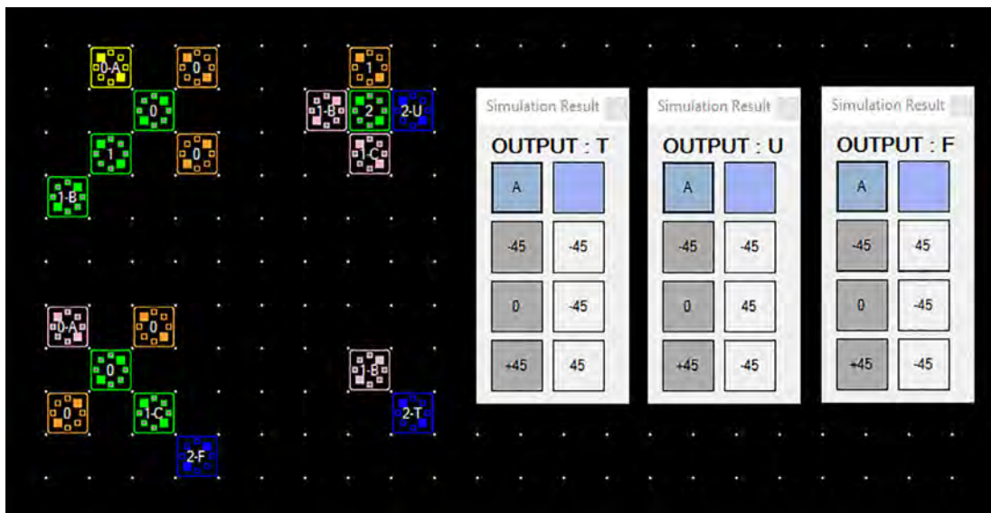
Fig. 8. Proposed ternary decoder and the related truth tables.
