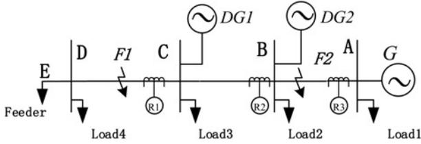
Fig. 2 Industrial distribution network with DG
