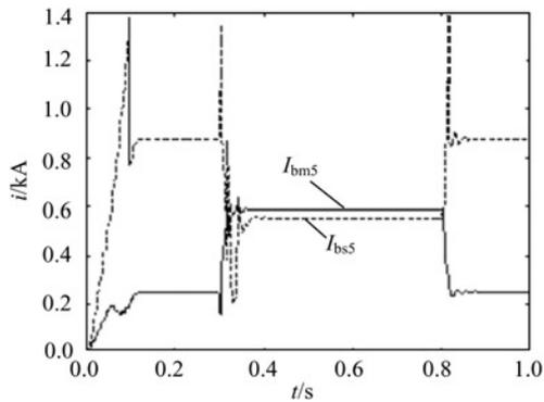
**Fig. 10** Characteristic curve of adaptive backup protection of the 5th relay when a phase-to-phase fault occurs on section AB close to bus B
