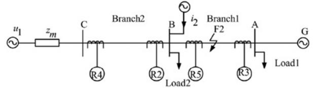
Fig. 5 Thevenin equivalent model behind the fourth relay
