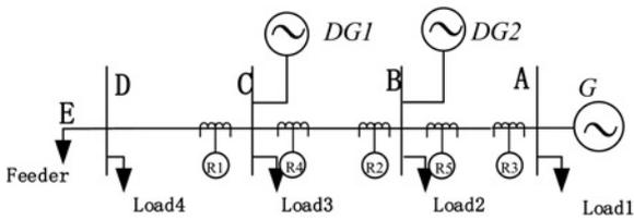
Fig. 3 Industrial distribution network with directional protection devices
