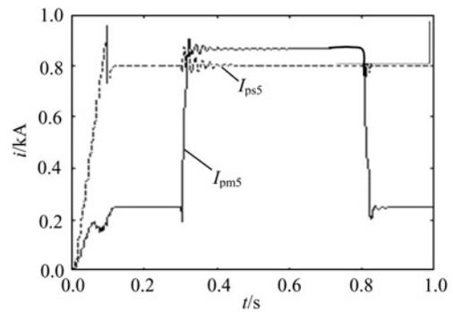
Fig. 7 Characteristic curve of adaptive primary protection of the 5th relay when a three-phase fault occurs in the middle of section BC
