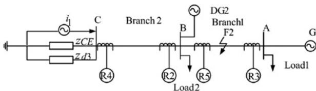
Fig. 4 Norton equivalent model behind the fourth relay
