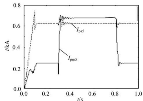
Fig. 8 Characteristic curve of adaptive primary protection of the 5th relay when a phase-to-phase fault occurs in the middle of section BC
