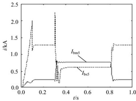
**Fig. 9** Characteristic curve of adaptive backup protection of the 5th relay when a three-phase fault occurs on section AB close to bus B
