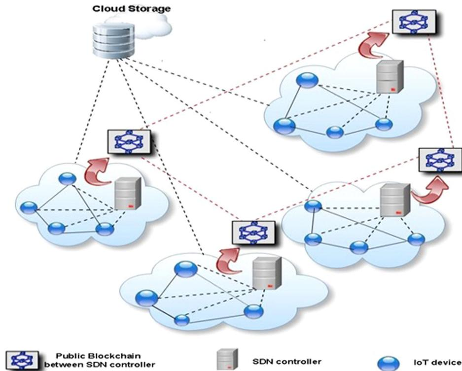
Fig. 1. Cluster-based proposed model with blockchain-enabled SDN controllers.
