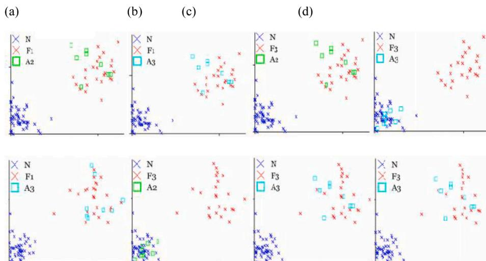
**Fig.: 2.** Simulation (first row) & Testbed (second row) Classification Areas for classifying attack instances on models trained with Normal and a Fault class. ) Classifying A2 instances on N & F1 model (b) Classifying A3 instances on N & F1 model (c) Classifying A2 instances on N & F3 model (d) Classifying A3 instances on N & F3 model.
