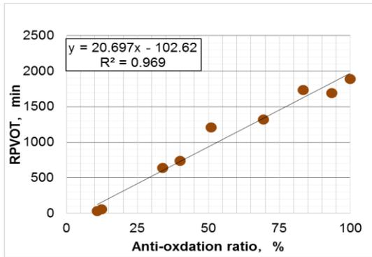
Figure 3. Relationship between the antioxidant ratio and the RPVOT value as measured in experimentally-deteriorated EMTO
