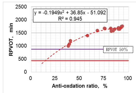
Figure 4. Relationship between the antioxidant ratio and the RPVOT value as measured in actually-used EMTO
