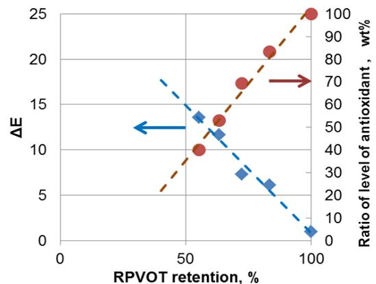
Figure 5. Relationship between RPVOT retention and  $\Delta E$ , and antioxidant ratio as measured in deteriorated EMTO
