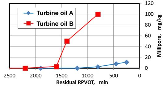
Figure 2. Relationship between the RPVOT value and the sludge formation
