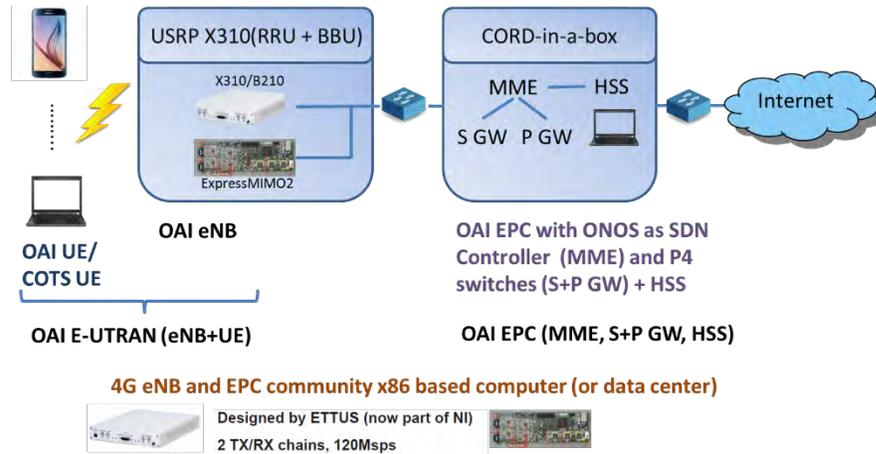
Figure 14 An OAI-based M-CORD Prototype at NCTU
