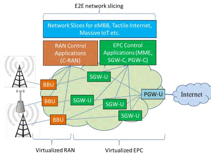
Figure 8 Realizing 5G network slicing by SDN/NFV
