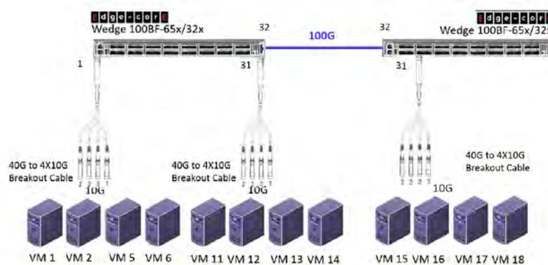
Figure 13 Topology of P4 testbed at NCTU
