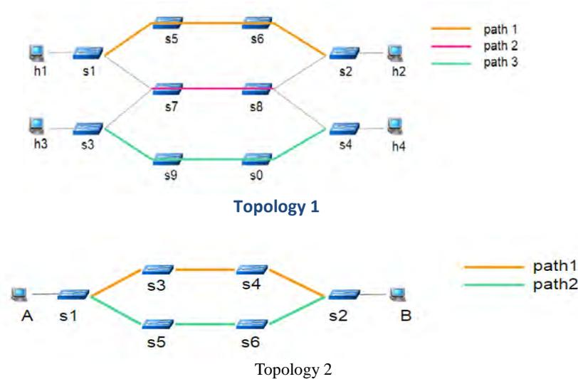
Figure 4(d) Topology1&2 for Dynamic Load Balancing and Congestion Avoidance
