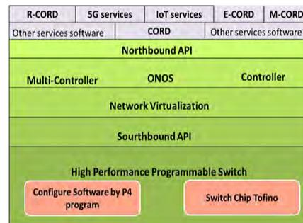
Figure 2(b) SDN Layered Architecture based on P4/ONOS/CORD
