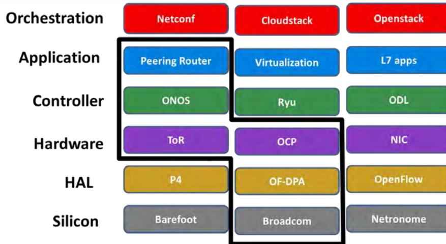
Figure 12 Solution: Vertically Integrated Stack as SDN Distribution
