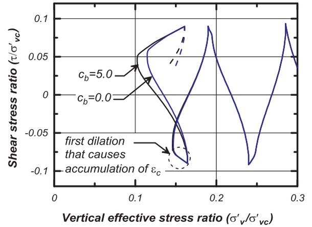
Fig. 3. Effects of input parameter  $c_b$  (fabric damage) on contraction rate.
