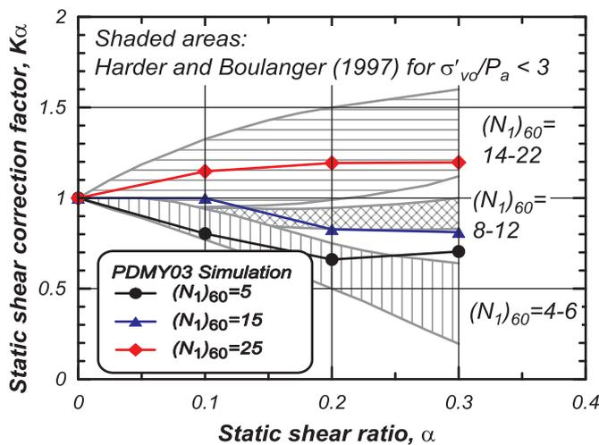
Fig. 13. Experimental trends for different  $(N_1)_{60}$  values and  $\sigma'_{vc} < 3$  atm from Harder and Boulanger [12] and model generated static shear stress correction factors ( $K_\alpha$ ) for  $\sigma'_{vc} = 1$  atm.
