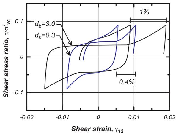
Fig. 7. Effects of input parameter  $d_b$  (fabric damage) on dilation rate.
