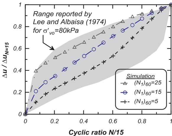
Fig. 10. Model predicted rate of pore pressure generation in DSS simulations for different relative densities at  $\sigma'_{vc} = 100 \text{ kPa}$  compared with the range expected from experimental observations.
