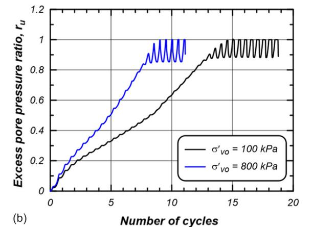
Fig. 4. Effects of overburden stress on contraction rate ( $K_\sigma$  effect) for input parameter  $c_c = 0.2$ ; (a) stress path and (b) pore water pressure ratio versus number of shear cycles.
