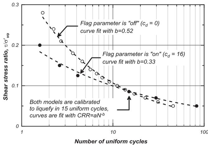
Fig. 5. Effects of input parameter  $c_d$  on the number of uniform loading cycles to trigger liquefaction.
