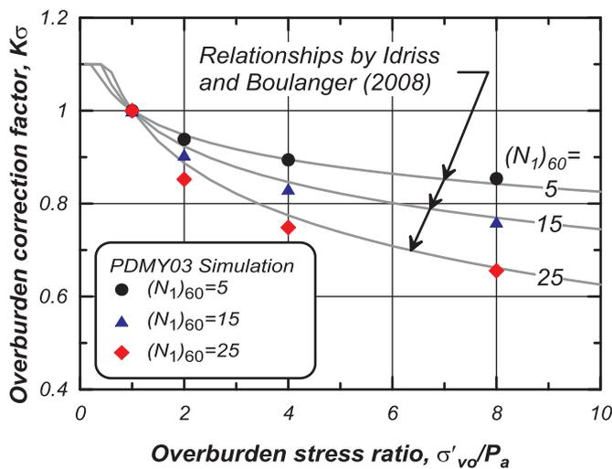
Fig. 12.  $K_\sigma$  relationships derived from model simulations compared to relationships by Idriss and Boulanger [14].
