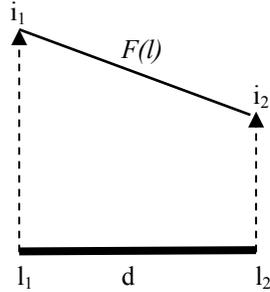
Fig. 2. Current distribution with ramp approximation
