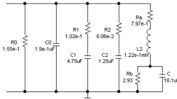
Fig 6. Circuit Synthesis for Counterpoise
