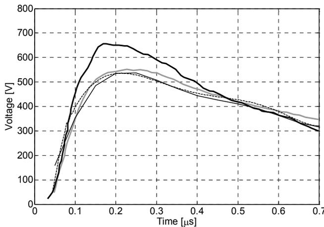
Fig. 10. Voltage at Injection Point - Counter poise. (Thick Black: Measurement, Gray: MM, Thin Black: HEM and Dashed: Synthesized).
