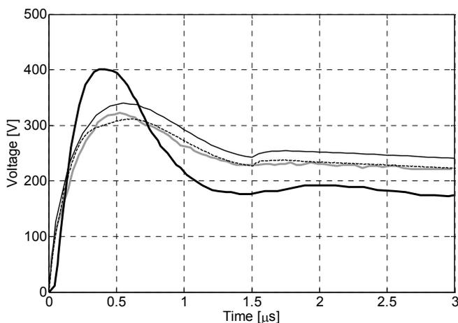
Fig. 11. Voltage at Injection Point - Rod. (Thick Black: Measurement, Gray: MM, Thin Black: HEM and Dashed: Synthesized).
