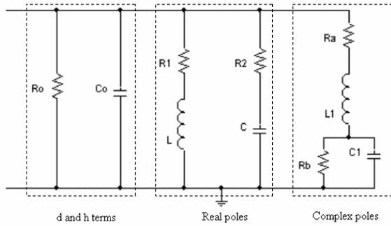
Fig 5. Circuit Synthesis Schematic
