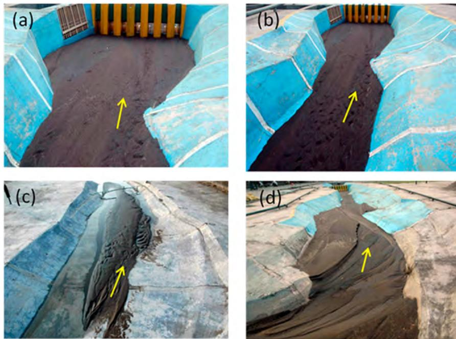
**Figure 9.** View of Punatsangchhu Reservoir model after flushing with  $1000 \text{ m}^3 \text{ s}^{-1}$  for 24 h.
