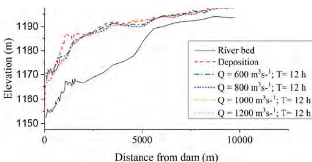
**Figure 10.** Longitudinal section of Punatsangchhu Reservoir after flushing for 12 h.
