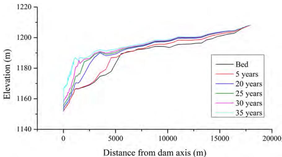
Figure 6. Longitudinal section profiles of reservoir bed after different years of reservoir operation.
