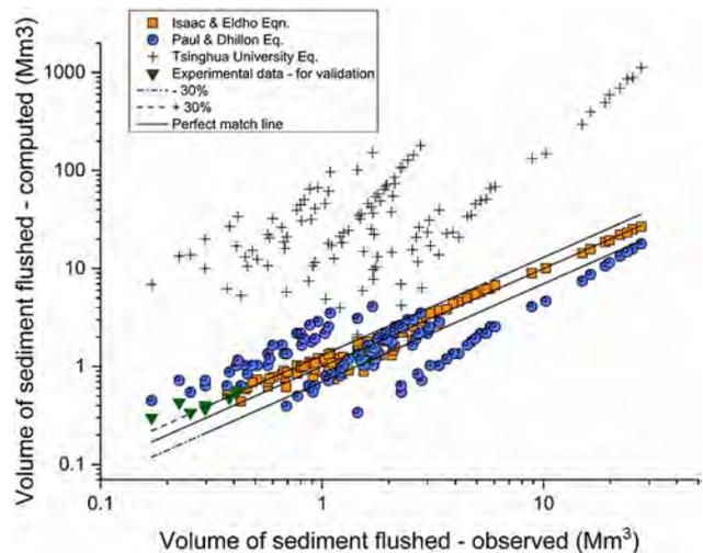
**Figure 15.** Comparison of observed and predicted values of the volume of sediment flushed ('moderate').
