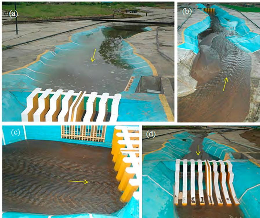
**Figure 8.** View of Punatsangchhu Reservoir model during flushing.
