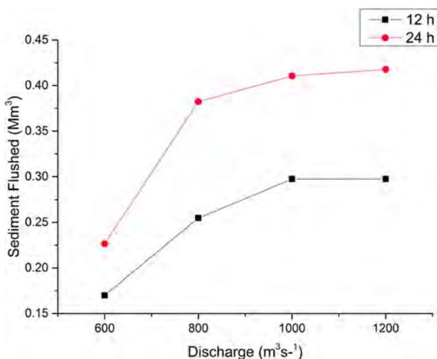
Figure 13. Volume of sediment flushed with different discharges for case study.
