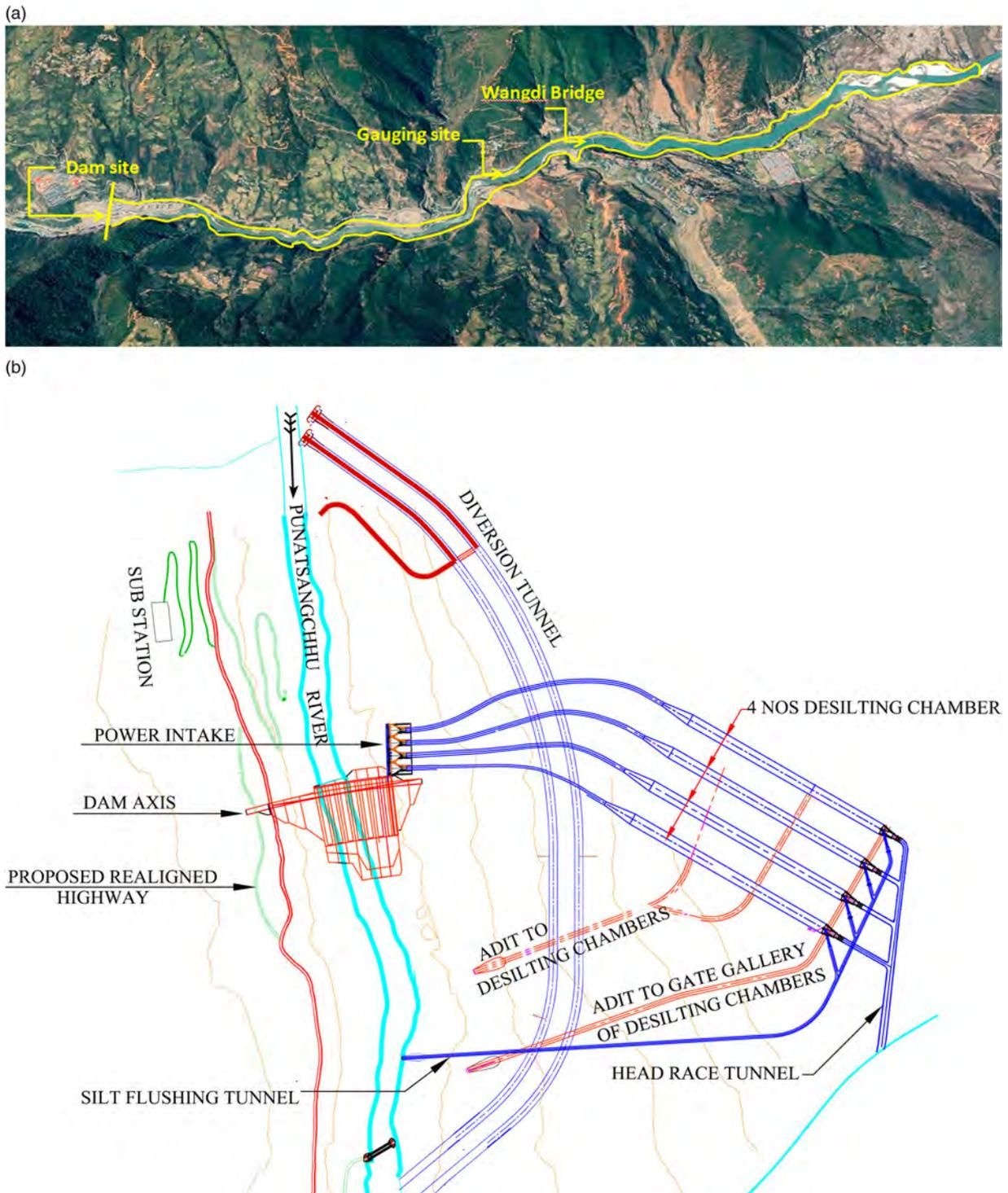
Figure 1. (a) Location map of the project. (b) General layout of the dam complex.
