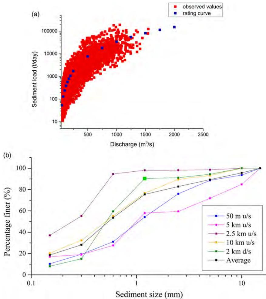
Figure 5. (a) The sediment rating curve. (b) Bed material gradation curves.
