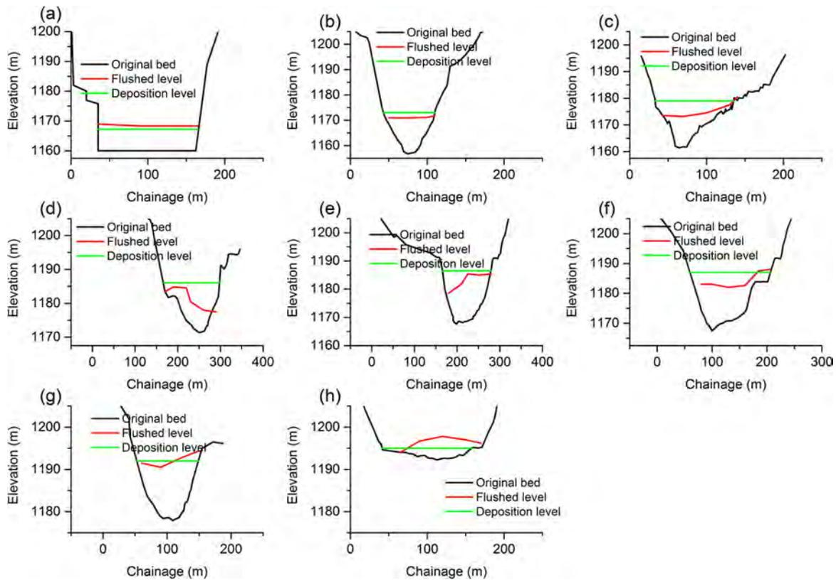
Figure 12. Typical cross-sections after flushing for 24 h with discharge of  $1000 \text{ m}^3 \text{ s}^{-1}$ .
