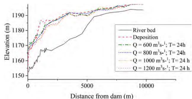
**Figure 11.** Longitudinal section of Punatsangchhu Reservoir after flushing for 24 h.
