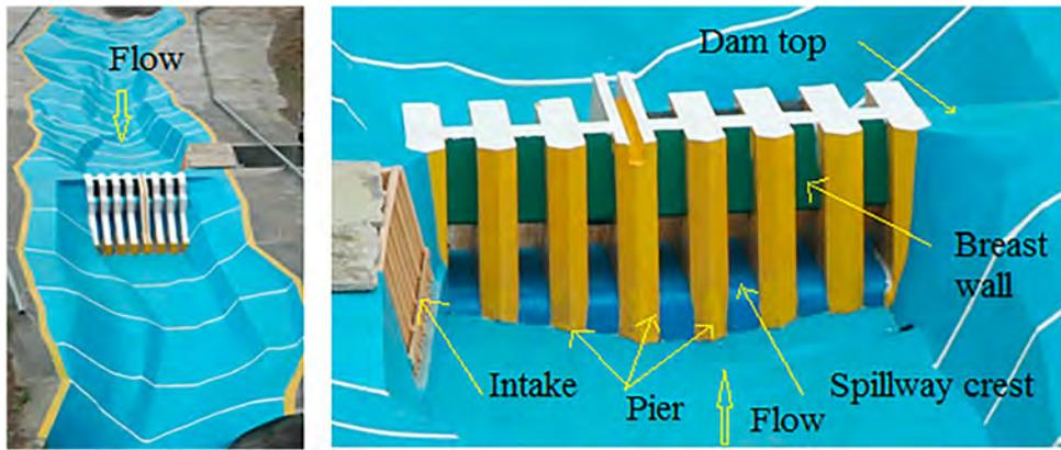
**Figure 7.** View of Punatsangchhu Reservoir model showing dam and spillway.
