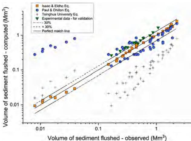
**Figure 14.** Comparison of observed and predicted values of the volume of sediment flushed ('steep').
