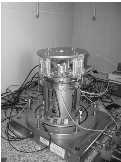
Fig. 1. Photography of GDS Resonant Column Apparatus with tested sample.
