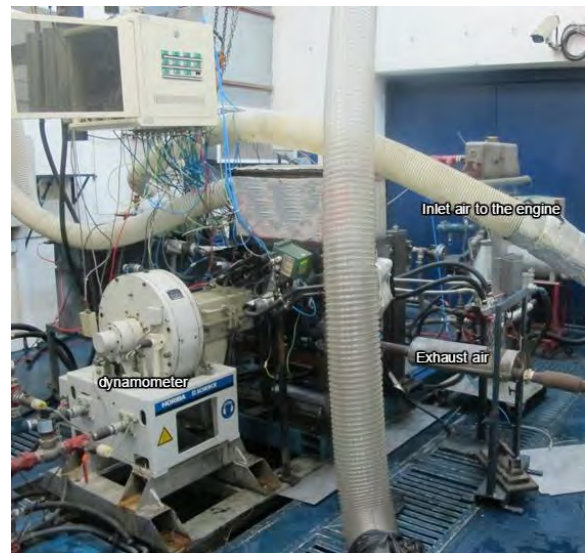
Figure 2a. A photograph of the experimental setup for measuring optimum engine temperature
