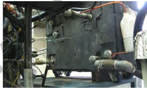
Figure 1: A photograph of the radiator submerged in a constant temperature pool in order to keep the radiator temperature constant
