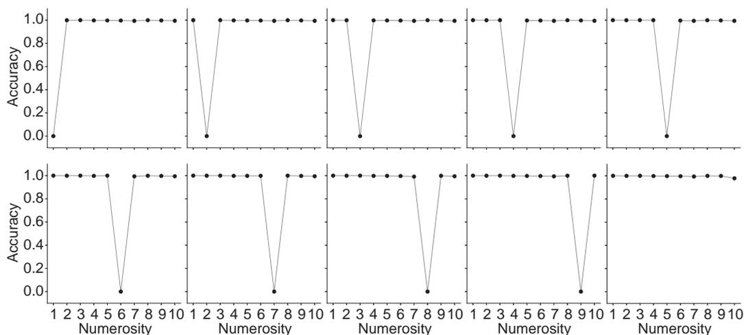
**Fig. 8.** Effect of silencing units in the hierarchical convolutional neural network (HCNN) selectively activating a particular output numerosity label. Single-numerosity classification accuracy of the HCNN is shown on the y-axis. When all the neural units selectively activating a single number label were silenced, the accuracy dropped to 0% for the silenced number, while the accuracy for all other numbers remained virtually unaffected in all cases.
