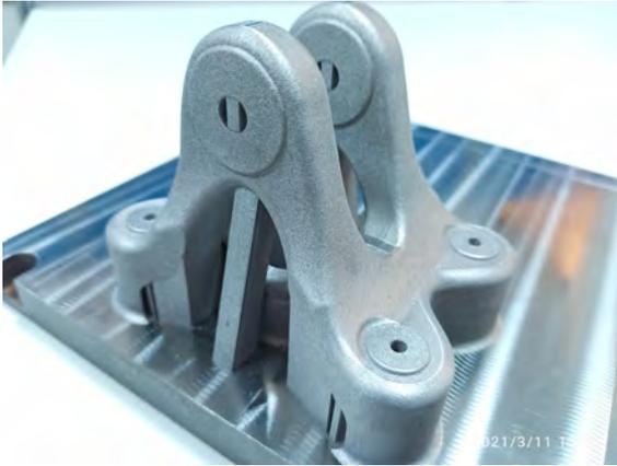
Fig. 9. L-PBF Manufactured optimized part
