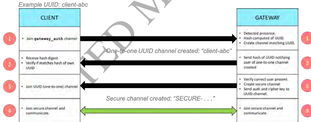
Figure 4: The four phases included within the three-step authentication process required to establish a secure communication channel
