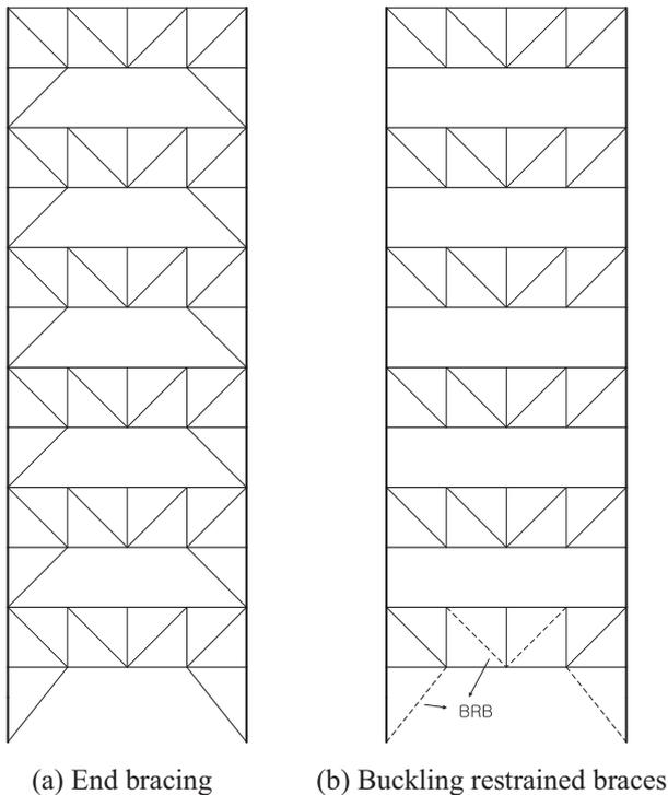
Fig. 20. Retrofit schemes for Type B structure.
