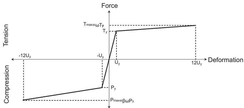
Fig. 22. Idealized backbone curve of the BRB.
