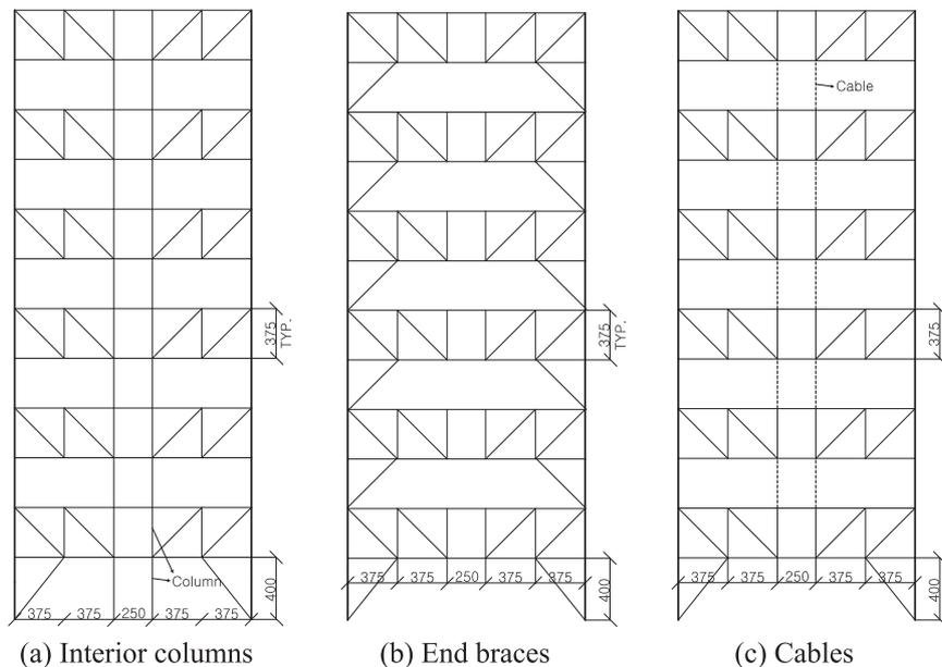
Fig. 14. Seismic reinforcing schemes for Type A structures.
