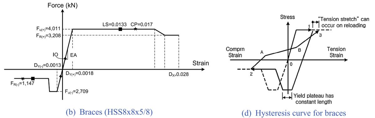
Fig. 4. Nonlinear force–displacement relationship of structural members.
