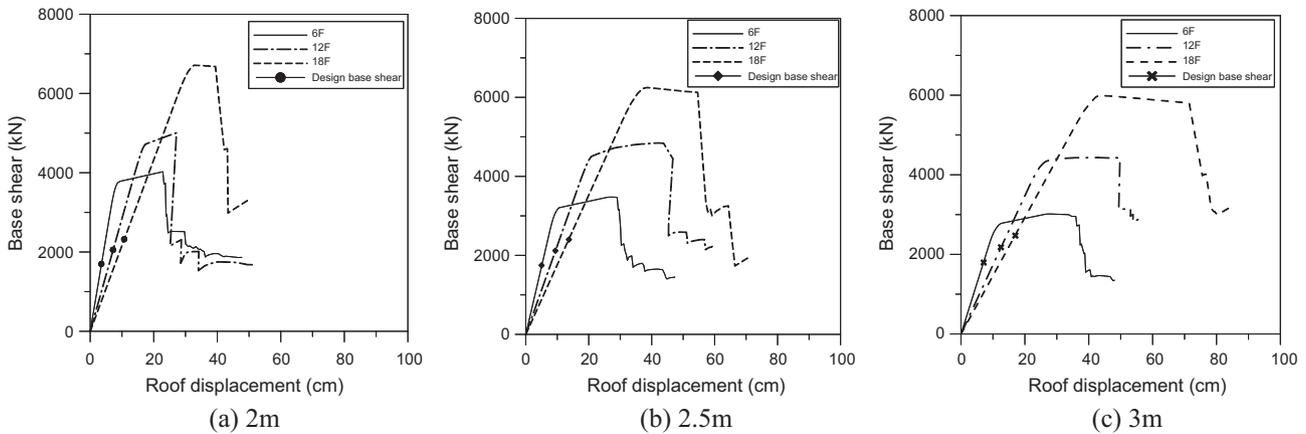
Fig. 5. Pushover curves of Type A STS model structures having viereindeel panels with different lengths.
