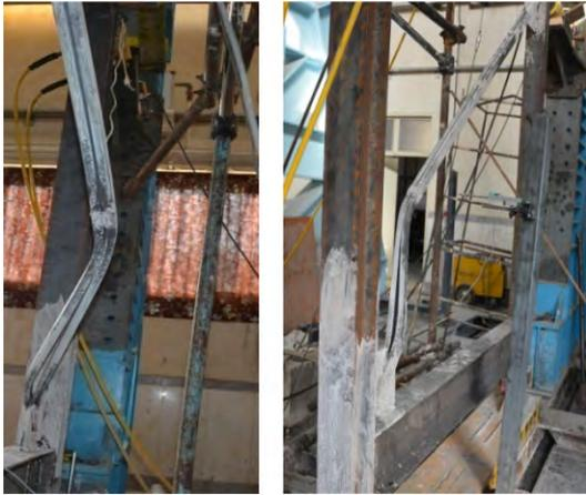
Figure 8. Large post buckling deformations in Test 2
