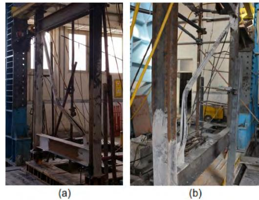
Figure 13. Deformations of braces (a) Test 1 (b) Test 2.
