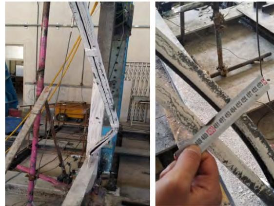
**Figure 6.** Large out-of-plane deformation of brace in Test 1.
