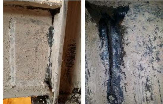
Figure 11. crack in connection of beam to column in test 3.
