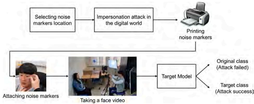
Fig. 1. The process of attacks by attaching noise markers on the face in the physical world.
