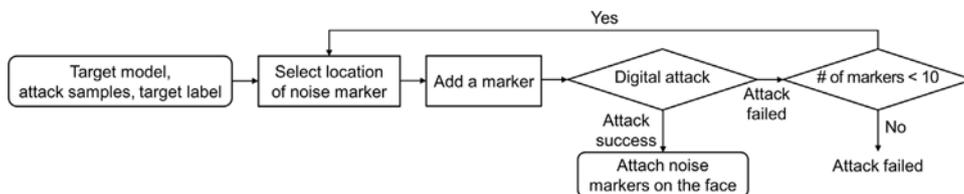
Fig. 6. The attack process to deceive deep FR models by attaching noise markers on the face in the digital environment.
