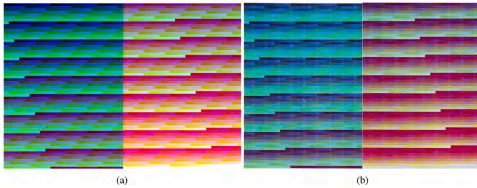
Fig. 4. The color mapping tables: (a) a color table on the digital environment, (b) a color table taken after printing. (For interpretation of the references to color in this figure legend, the reader is referred to the web version of this article.)
