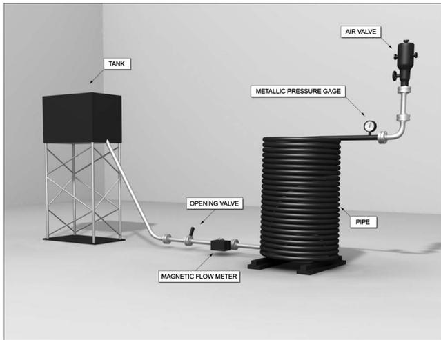
Fig. 2. Three-dimensional schematic of laboratory model
