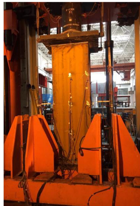
Fig. 7. The axial compression test equipment.
