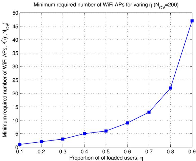
Fig. 7. Minimum required Number of WiFi APs for varying  $\eta$  ( $N_{OV} = 200$ )
