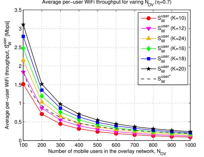
Fig. 4. Average per-user WiFi throughput for varying  $N_{OV}$  ( $\eta = 0.7$ )
