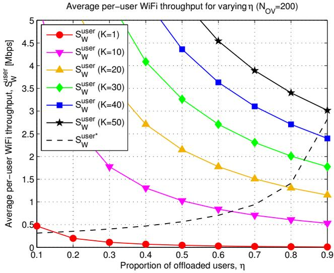
Fig. 6. Average per-user WiFi throughput for varying  $\eta$  ( $N_{OV} = 200$ )
