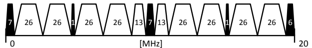
Fig. 2. Illustration of OFDMA as specified in IEEE 802.11ax. The numbers represent the amount of sub-carriers allocated for each resource unit. Unused sub-carriers are indicated with black.
