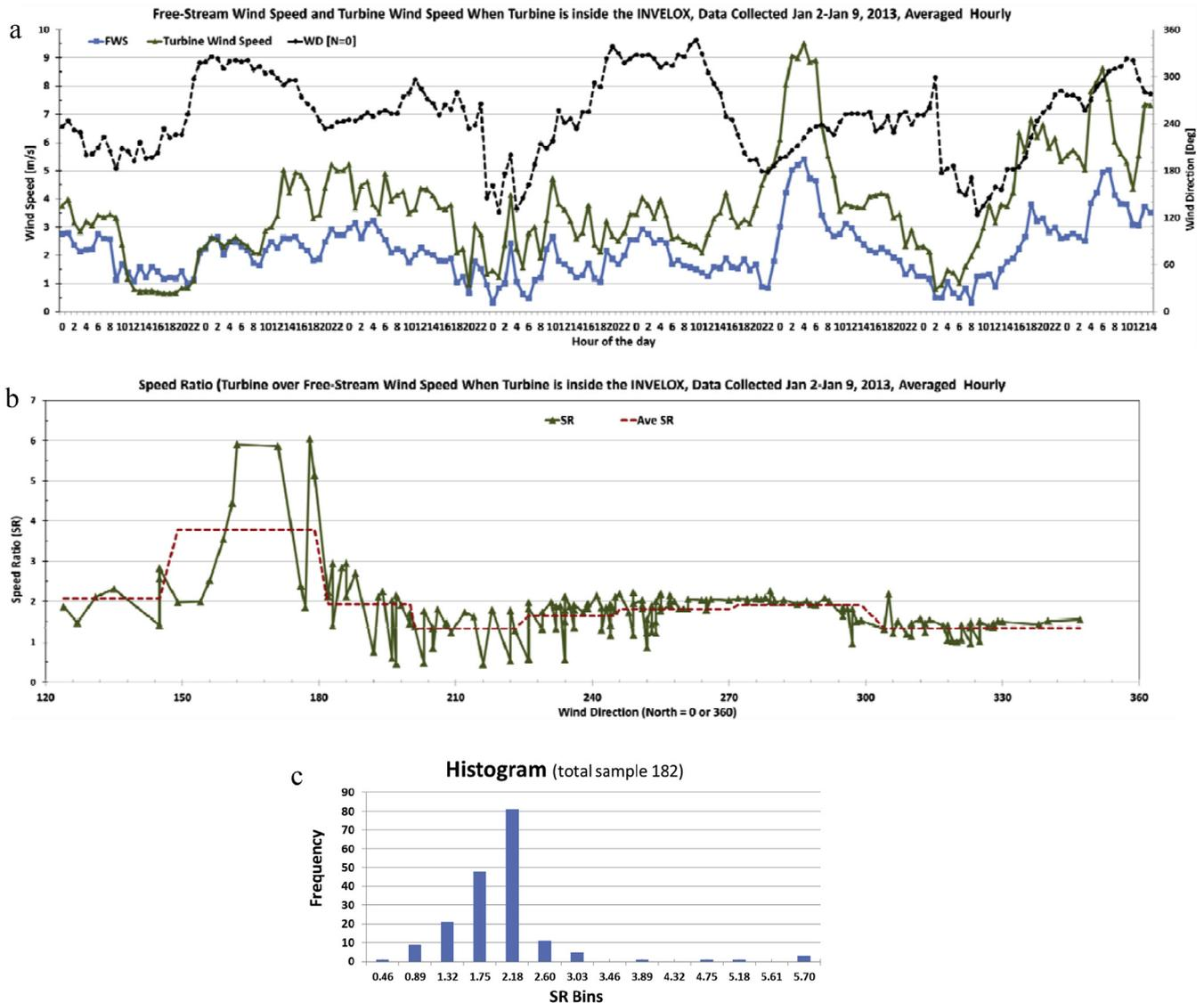
**Fig. 9.** (a) Free stream and turbine wind speed and wind direction for data measured over 8 days. (b) Speed ratio (turbine over free stream wind speed) versus wind direction for data measured over 8 days. (c) Histogram/frequency of appearance analysis of speed ratio SR data shown in Fig. 9a and b, average value of SR is 1.81 and most probable value is 2.18.
