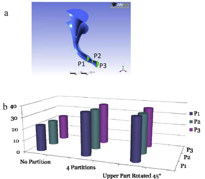
Fig. 6. (a) Locations along the Venturi section where mass flow rate was computed. (b) Comparison of captured mass flow rate (kg/s) by different intake configurations.
