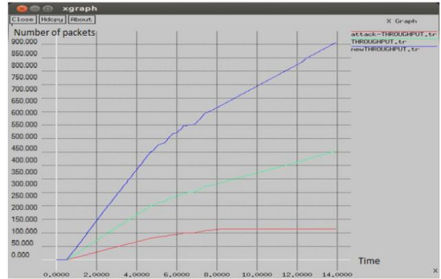
Figure 7. Comparison of LEACH, attack and proposed technique in terms of throughput
