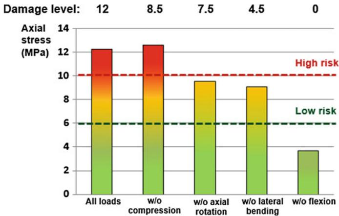
**Fig. 3** Axial stress generated in the PL-1 section in the caudal region in the five loading conditions. In the *upper part* the recurring of AFF is indicated, whereas in the *lower part* the risk failure of the group is written
