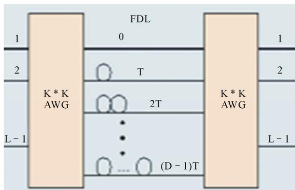
**Figure 5. Wavelength routing based optical packet buffer.**
