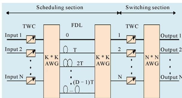
**Figure 6.** Input buffered optical packet switch.
