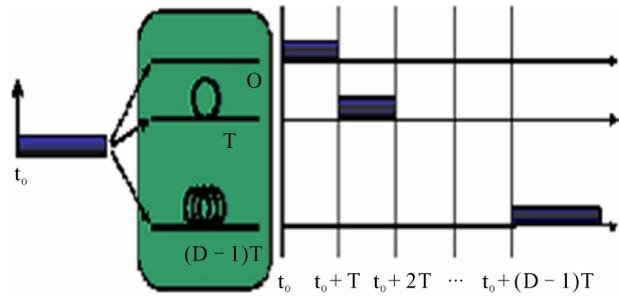
**Figure 1.** An optical buffer based on fiber delay lines.
