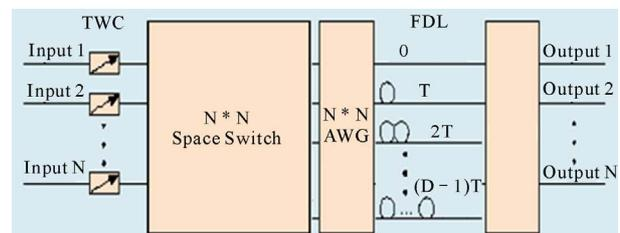
**Figure 7.** Output buffered switch architecture.
