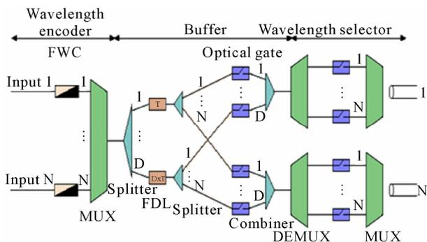
**Figure 3. Broadcast-and-select switch architecture with N ports, W wavelengths, and D FDLs.**
