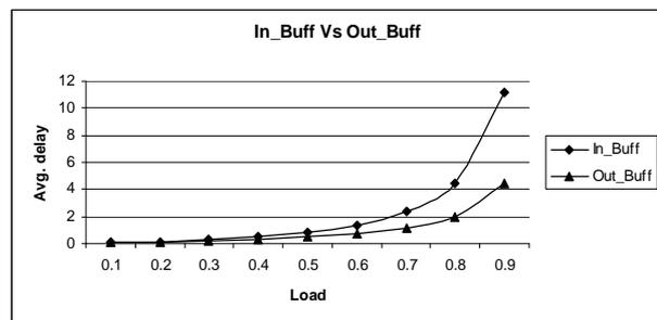
Figure 11. Delay versus offered load for input buffered and output buffered architectures for switch size  $N = 64$  and number of FDLs,  $D = 64$ .
