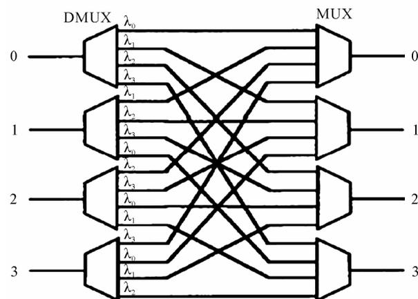
**Figure 4. 4 \* 4 arrayed-waveguide grating (AWG) multiplexers.**
