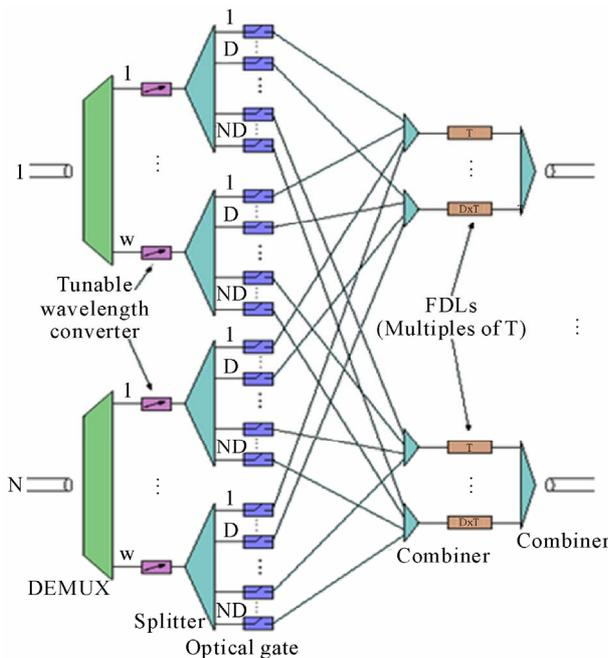
**Figure 2.** Space switch architecture with  $N$  ports,  $W$  wavelengths, and  $D$  FDLs.
