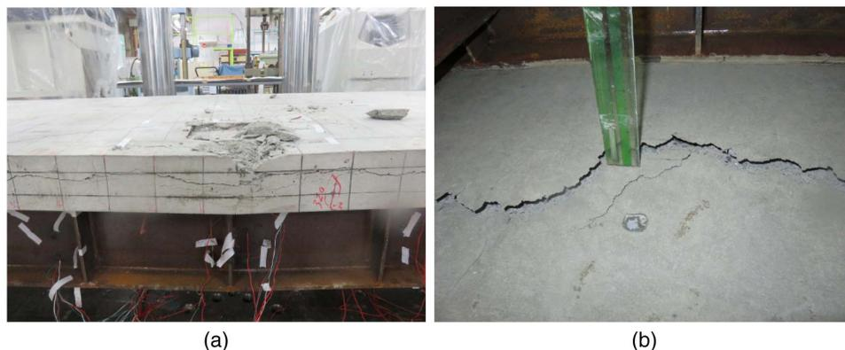
Fig. 8. Failure mode of the test specimen: (a) top view; and (b) bottom view of the concrete slab.
