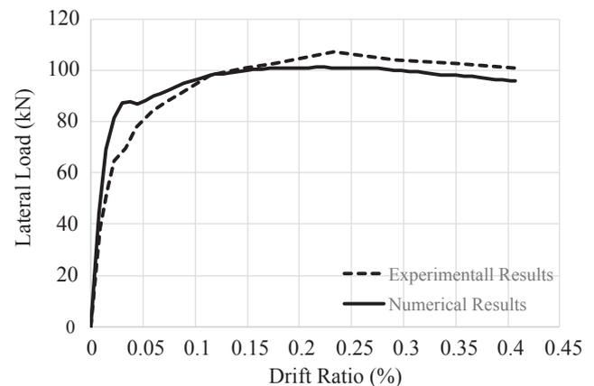
Fig. 4. Experimental vs Numerical results for unreinforced brick masonry structure.
