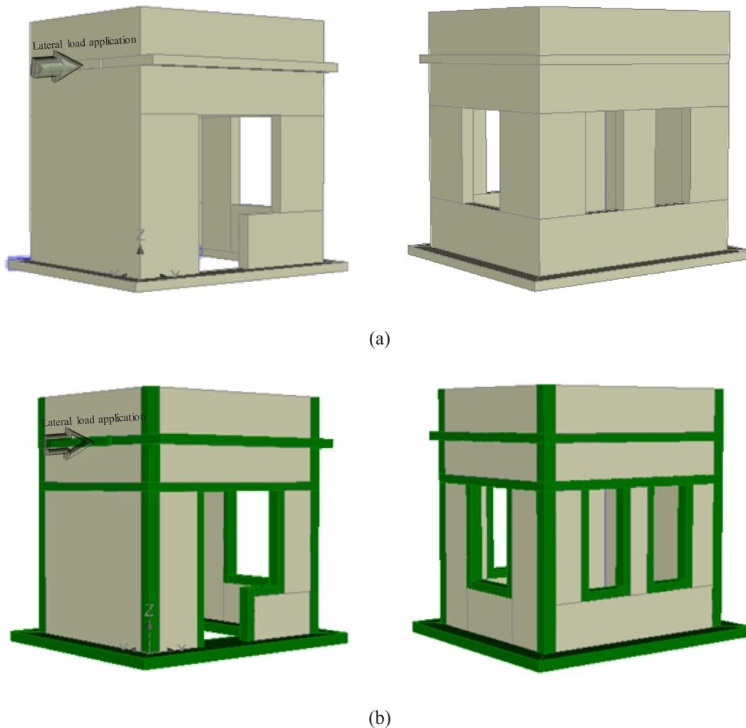
Fig. 3. Macro-element modeling details of (a) unreinforced masonry and (b) confined masonry structures.
