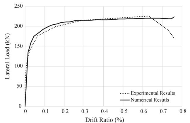
Fig. 7. Experimental vs Numerical curve for confined brick masonry structure.
