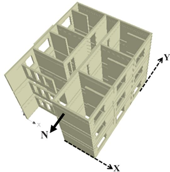
Fig. 9. Three dimensional computational model of a typical three story building structure.
