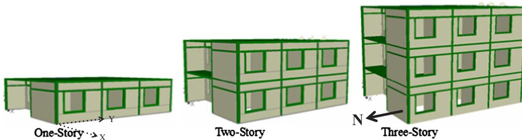
Fig. 15. Confined masonry solution for all three story levels (showing X (transverse) and Y (longitudinal) directions).
