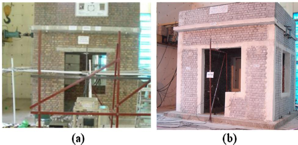
Fig. 2. Full scale masonry structure (a) unreinforced masonry [39], (b) confined masonry [40].
