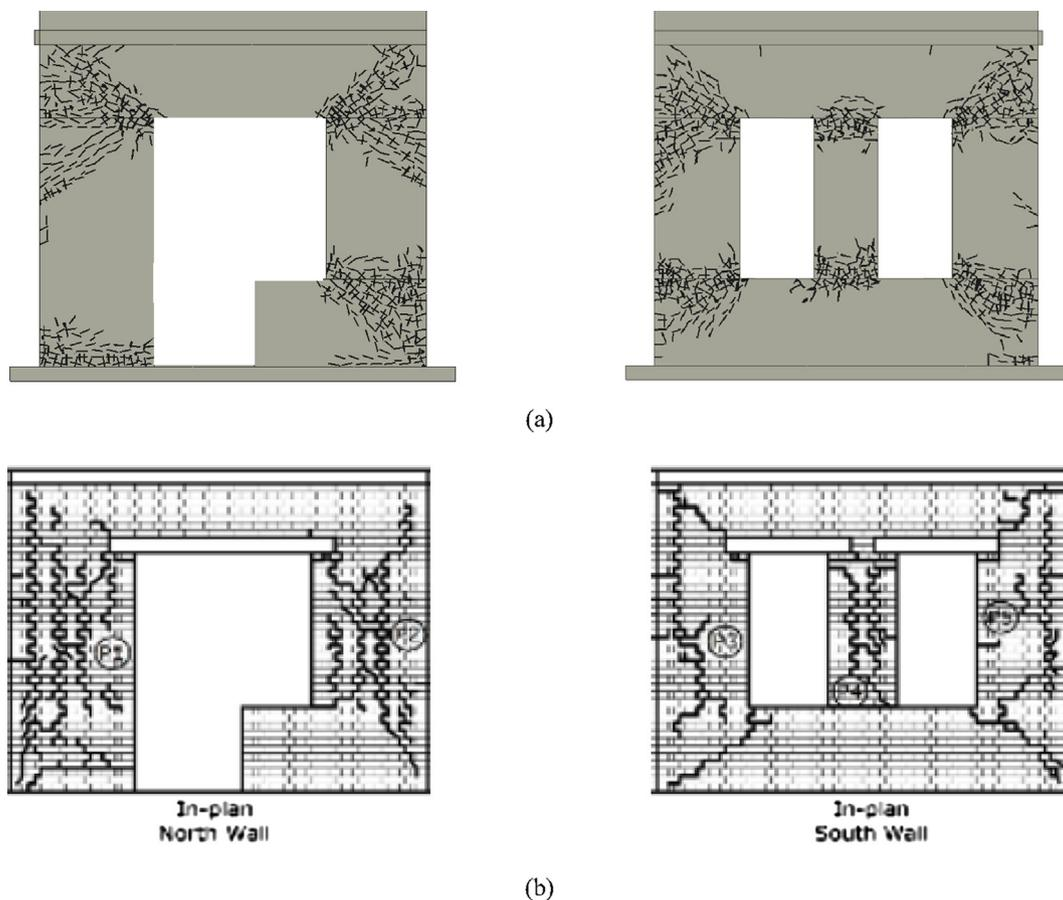
Fig. 5. Comparison of (a) Numerical and (b) Experimental Damage Patterns of URM.
