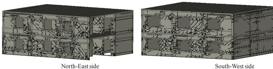
Fig. 17. Damage Mechanism of double story confined masonry structure.
