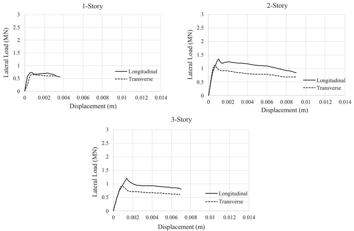
Fig. 14. Pushover curves for unreinforced masonry structures in X (transverse) and Y (longitudinal) directions.
