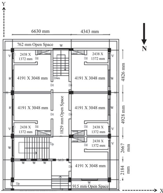
Fig. 8. Plan details (Ground floor) of the case study buildings, showing X (transverse) and Y (longitudinal) directions.
