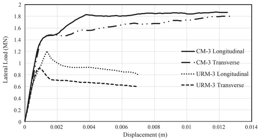
Fig. 22. Comparison of triple story structures for confined and unreinforced masonry solutions.
