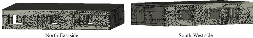
Fig. 16. Damage Mechanism of single story confined masonry structure.
