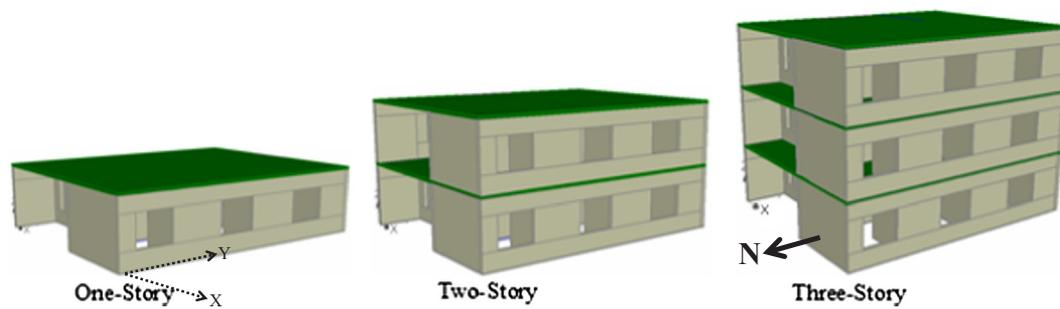
Fig. 10. Unreinforced masonry solution for all three story levels (showing X (transverse) and Y (longitudinal) directions).
