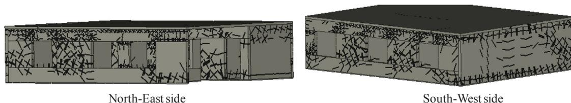
Fig. 11. Damage Mechanism of single story unreinforced masonry structure.
