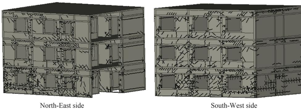
Fig. 18. Damage Mechanism of triple story confined masonry structure.
