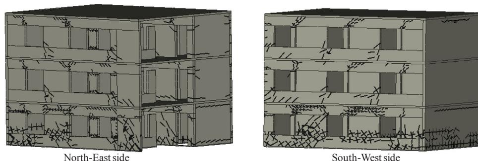
Fig. 13. Damage Mechanism of triple story unreinforced masonry structure.
