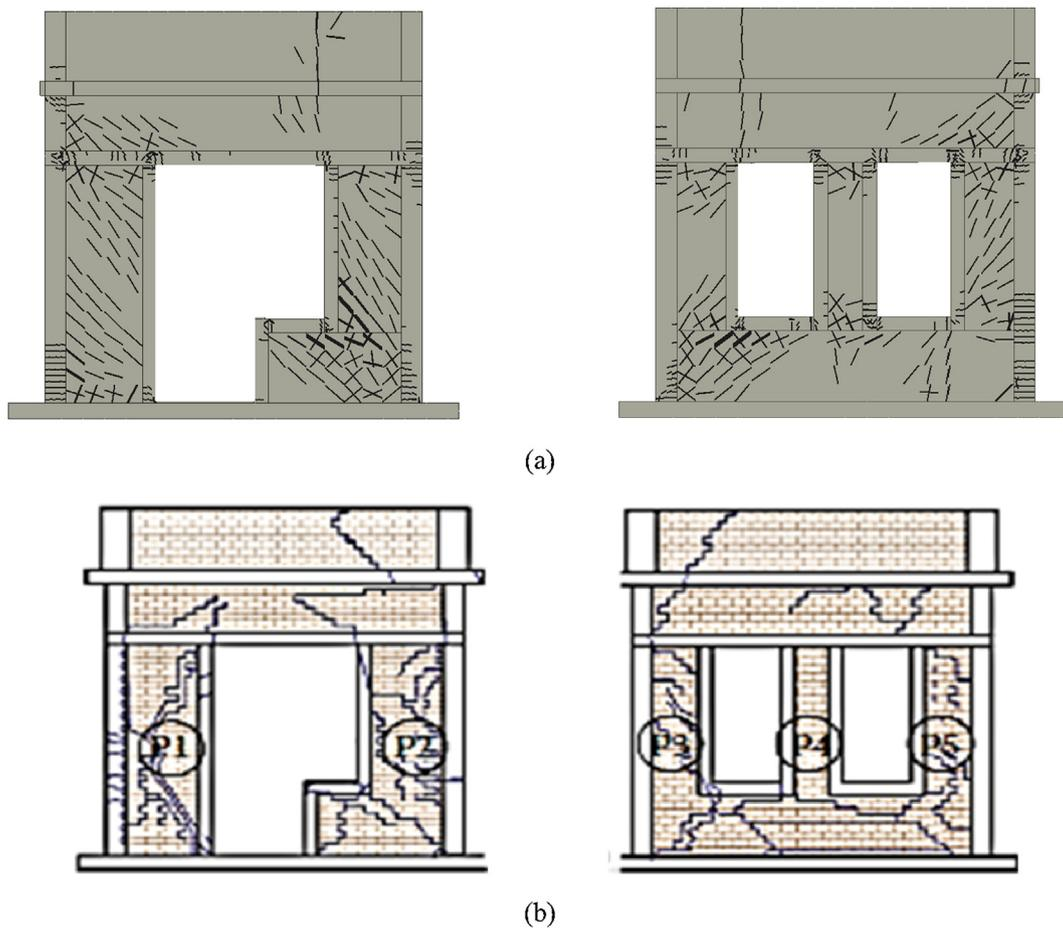
Fig. 6. Comparison of (a) Numerical and (b) Experimental Damage Patterns of CM.
