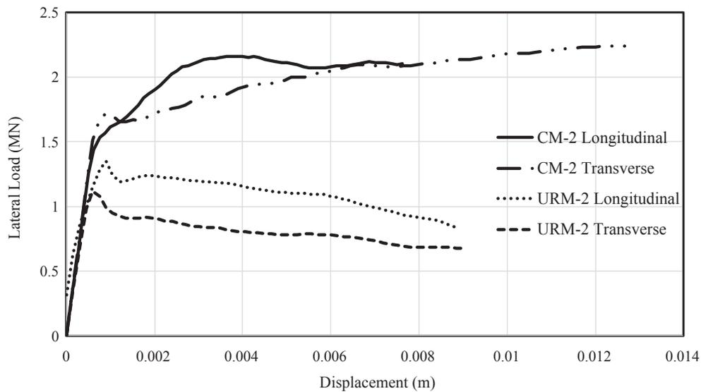
Fig. 21. Comparison of double story structures for confined and unreinforced masonry solutions.
