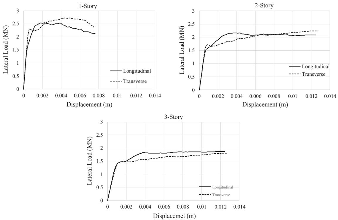
Fig. 19. Pushover curves for confined masonry structures in X (transverse) and Y (longitudinal) directions.
