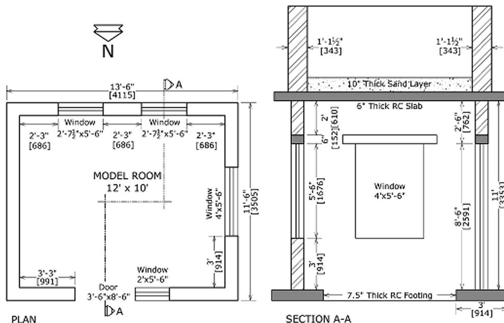
Fig. 1. Structure Details (dimensions in brackets are in mm) [39].
