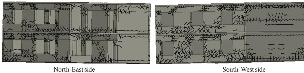
Fig. 12. Damage Mechanism of double story unreinforced masonry structure.
