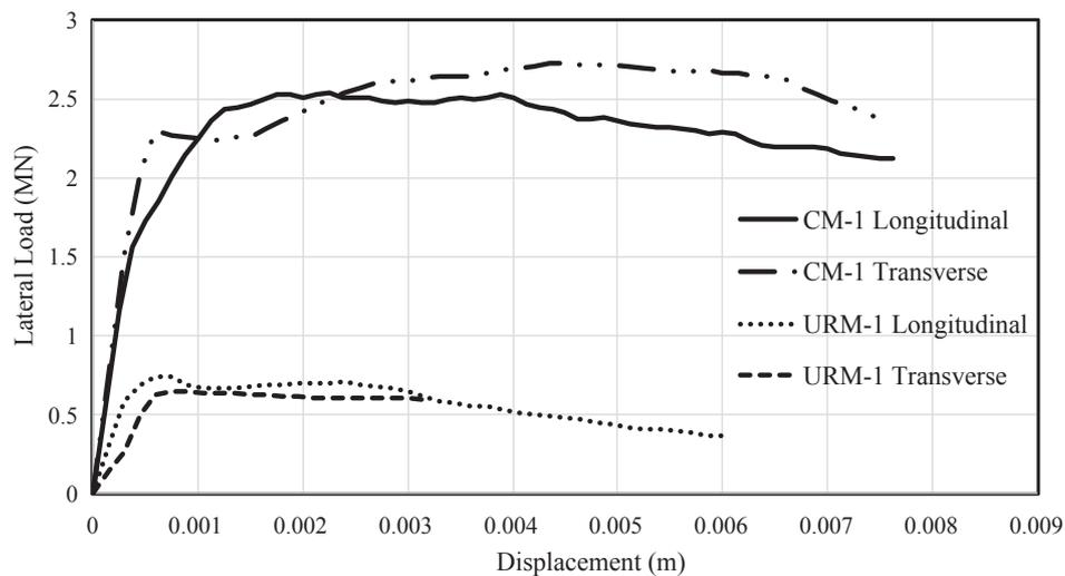
Fig. 20. Comparison of single story structures for confined and unreinforced masonry solutions.
