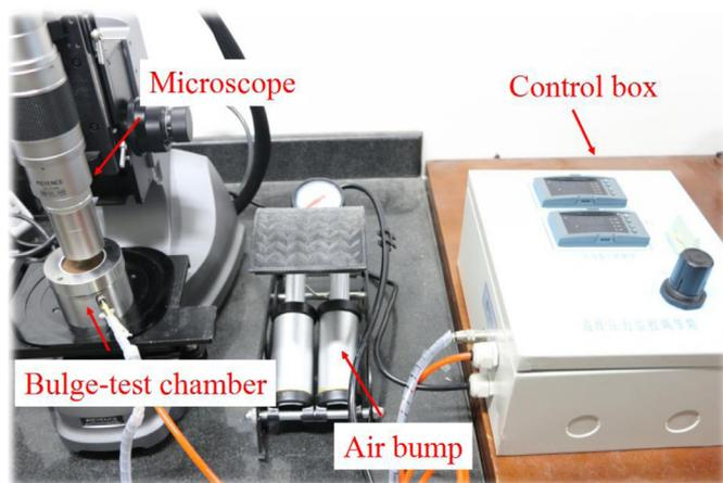
Fig. 6. The bulge-test system, including a control box, an air bump, a microscope and a bulge-test chamber.
