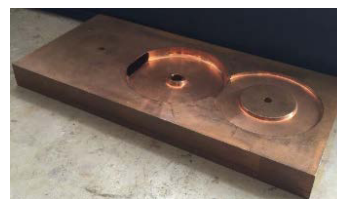
Fig. 3. OHFC 99.99% copper back-to-back cell after the brazing process
