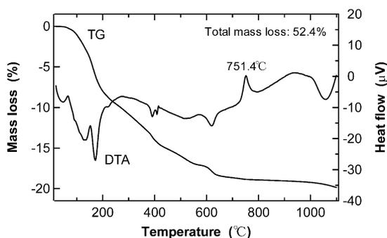
Fig. 1. TG–DTA curves of gel powder dried at 100 °C for 24 h.
