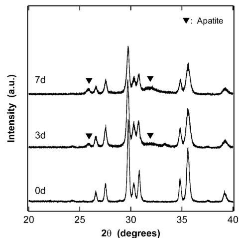
Fig. 5. X-ray diffraction patterns of the outer surface of diopside pellets sintered at 1100 °C for 2 h before and after their immersion in SBF for each soaking time.
