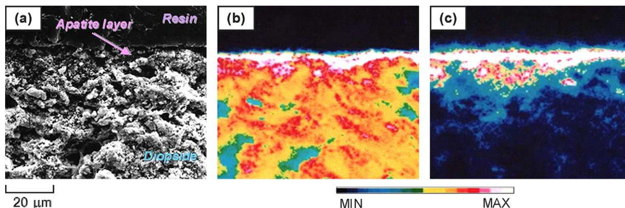
Fig. 6. EPMA images of the polished cross-section of diopside pellet sintered at 1100 °C for 2 h after its immersion in SBF for 7 days: SEM photograph (a), Ca (b) and P (c) element distribution maps.
