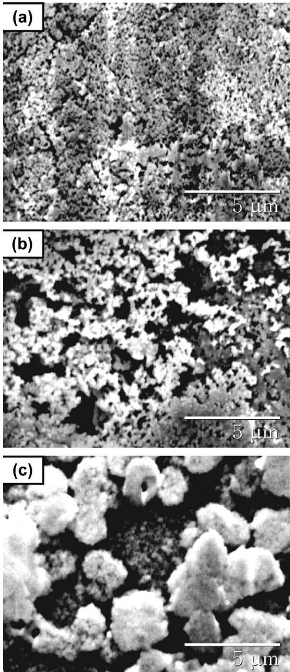
Fig. 4. SEM microphotographs of the outer surface of diopside pellets sintered at 1100 °C for 2 h before (a) and after their immersion in SBF for 3 days (b) and 7 days (c), respectively.
