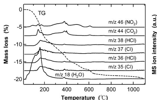
Fig. 3. TG–MS curves of gel powder dried at 100 °C for 24 h.
