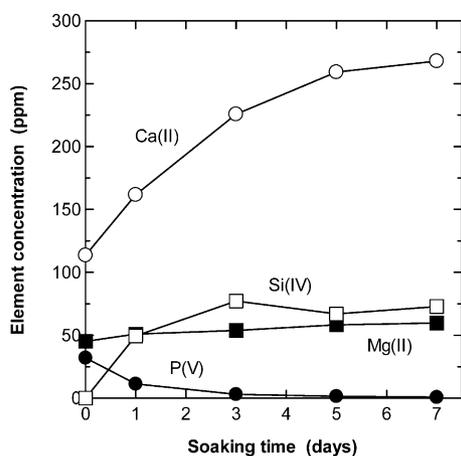
Fig. 7. Changes in element concentrations of SBF as a function of soaking time of diopside pellets sintered at 1100 °C for 2 h.
