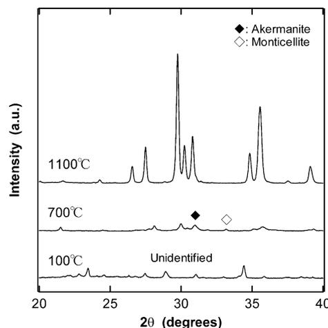
Fig. 2. Powder X-ray diffraction patterns of gel powder heated at various temperatures.
