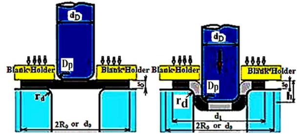
Fig. 2. Changing of the dimensions, over punch stroke in cup deep drawing processes
