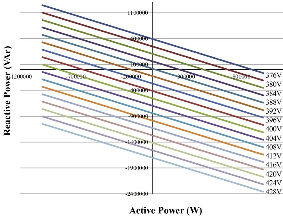
Fig. 4. Relationship between active power flow and reactive power flow under various regulated voltage levels.
