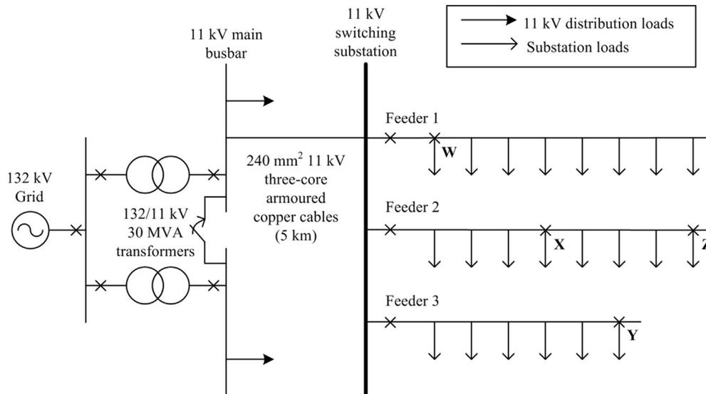
Fig. 2. Single-line diagram of the generic test network.
