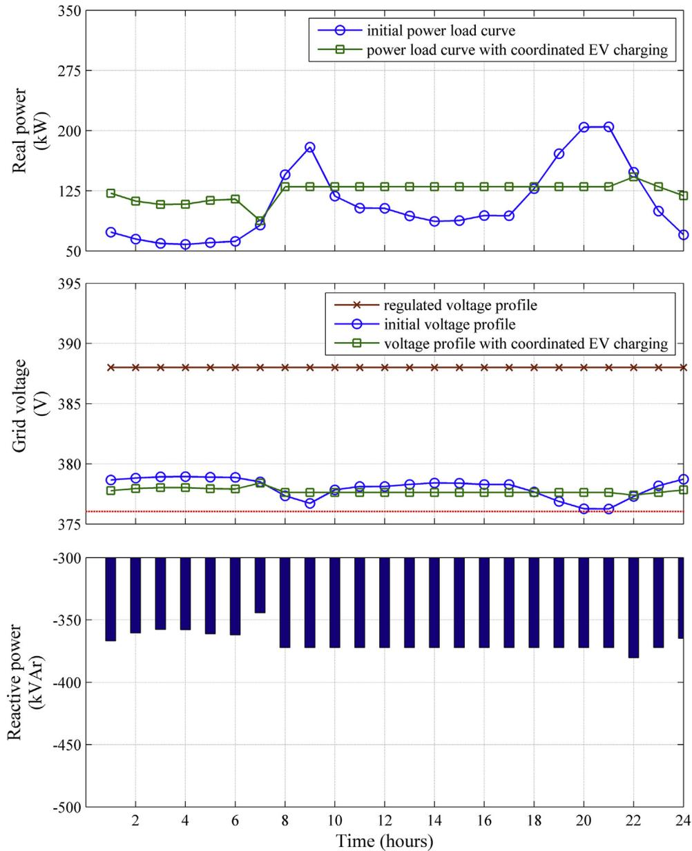
Fig. 11. Results of coordinated EV charging with voltage regulation.
