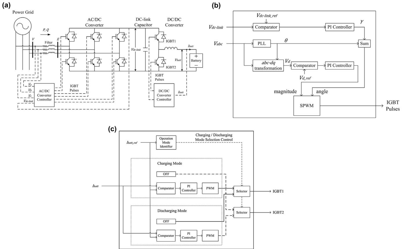
Fig. 1. Proposed grid-connected bidirectional V2G charger: (a) Configuration of the V2G charger, (b) controller of the AC/DC converter and (c) controller of the DC/DC converter.
