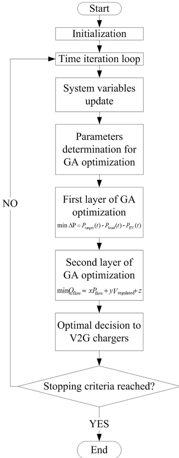
Fig. 7. Flow chart of V2G optimization algorithm.
