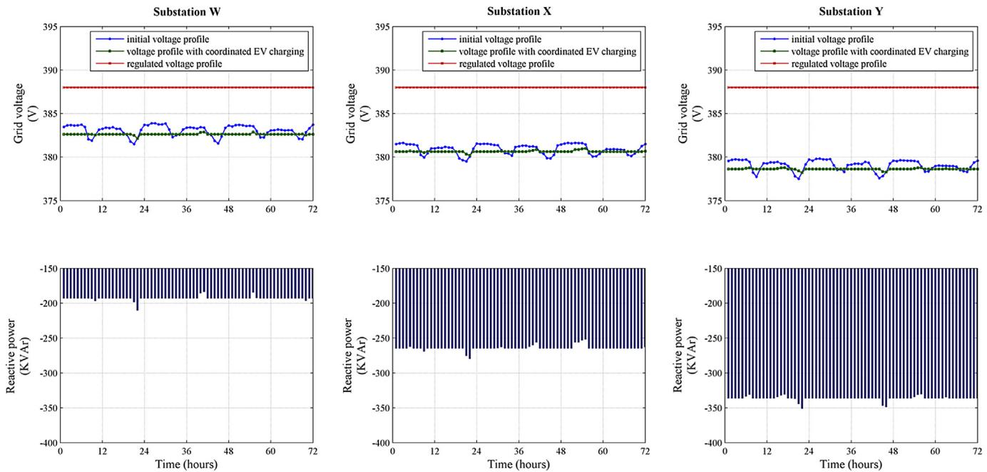
Fig. 14. Voltage profiles and the supplied reactive power by the V2G chargers at substations W, X and Y.
