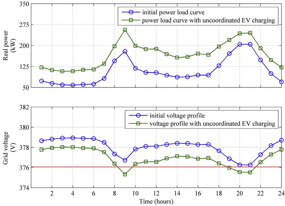
Fig. 8. Results of uncoordinated EV charging without voltage regulation.
