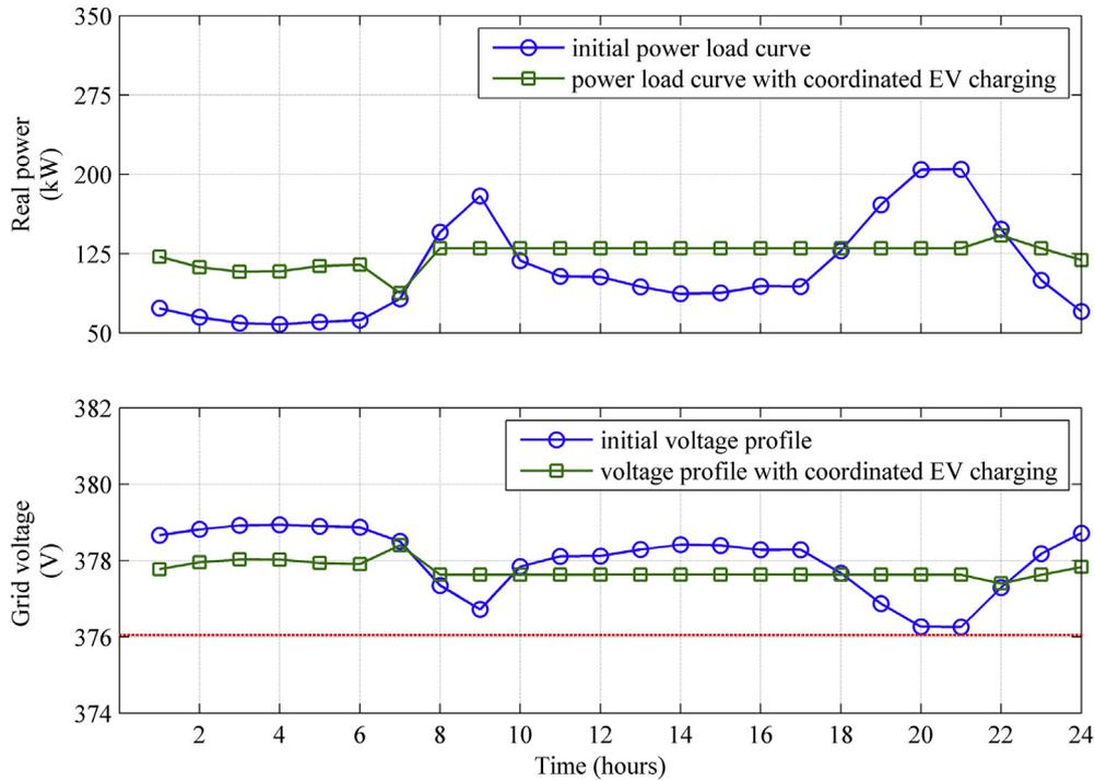
Fig. 9. Results of coordinated EV charging without voltage regulation.
