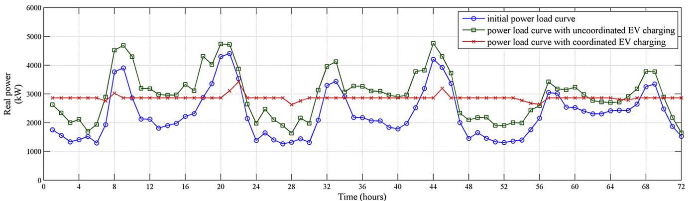
Fig. 13. Comparison of the initial and optimal power load curves at the 11 kV switching substation.
