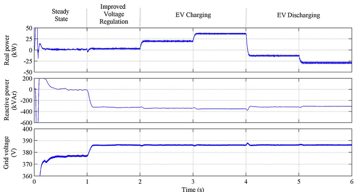
Fig. 3. Simulation results of real power flow, reactive power flow and grid voltage.
