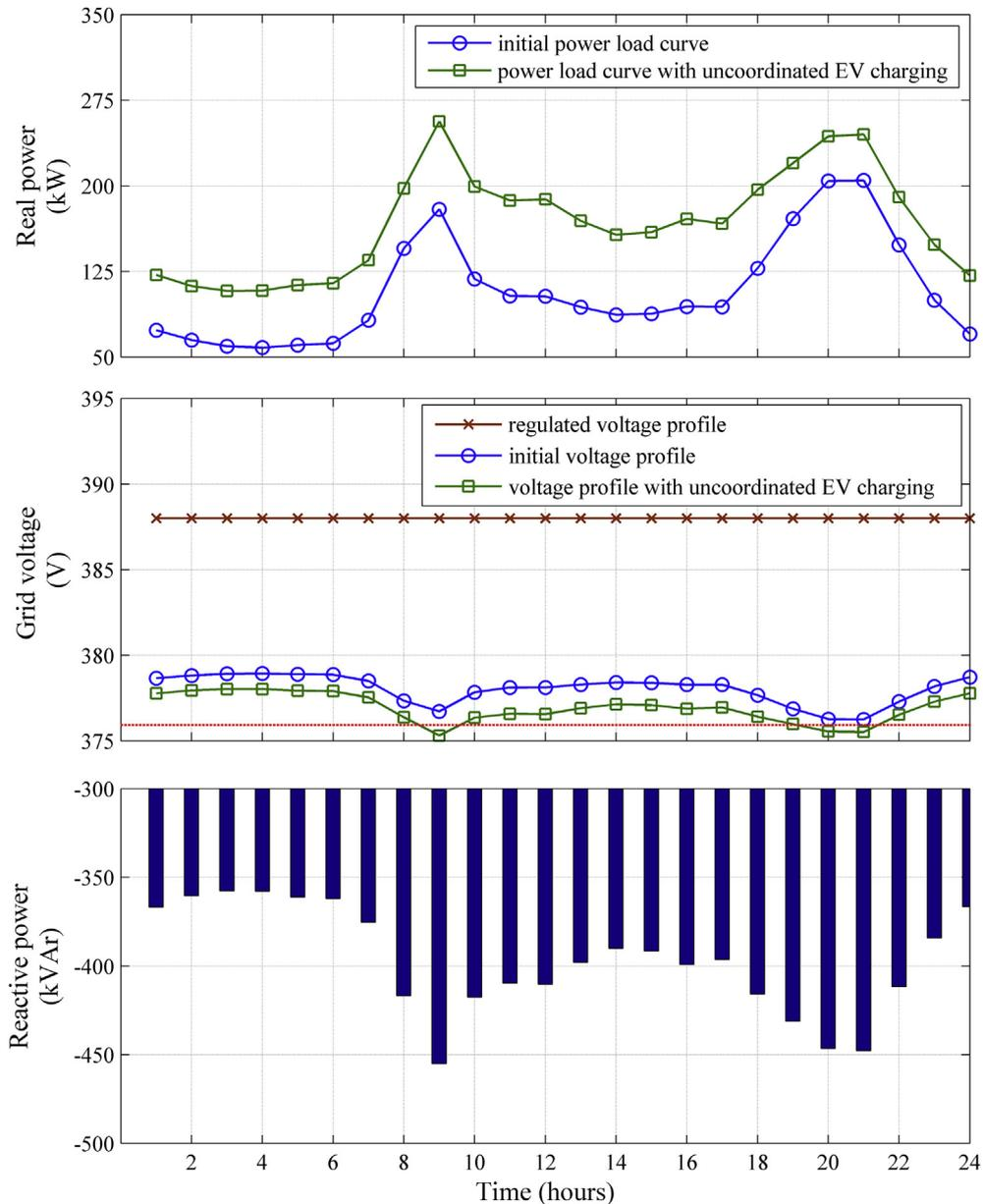
Fig. 10. Results of uncoordinated EV charging with voltage regulation.
