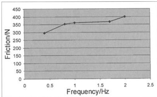
Figure 6 : Friction variation with speed
