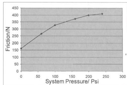
Figure 4 : Max friction for varying input pressures
