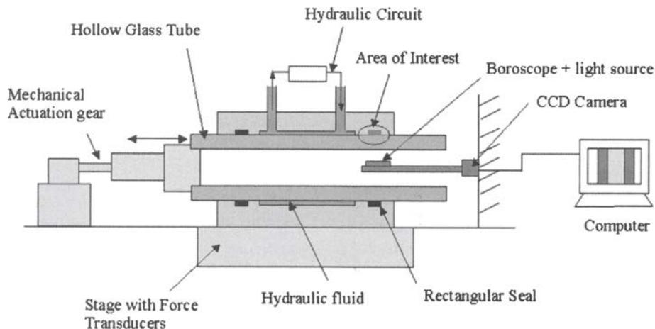
Figure 1 : General layout of seal specific rig
