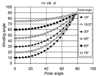
Figure 6: Sphere winding angle as a function of the polar angle.
