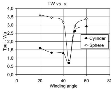
Figure 4: Influence of the winding angle. TW coefficient vs. Winding angle.
