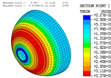
Figure 8: Tsai–Wu coefficient behavior on the sphere. Initial winding angle 45°.
