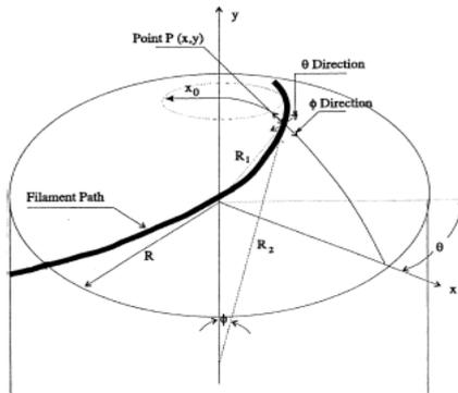
Figure 5: Helical winding in spherical dome vessel. Geodesic path.
