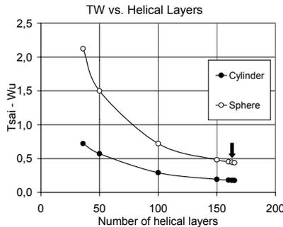
Figure 9: Influence of the number of helical layers on Tsai – Wu coefficient.
