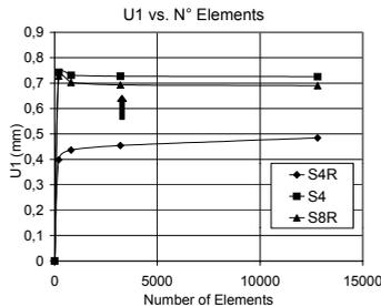
Figure 1: Comparison of the element types. Displacement 1 vs. Number of elements.
