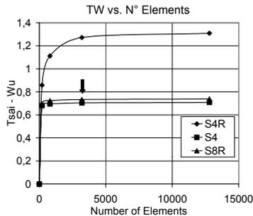
Figure 3: Comparison of the element types. TW coefficient vs. Number of elements.
