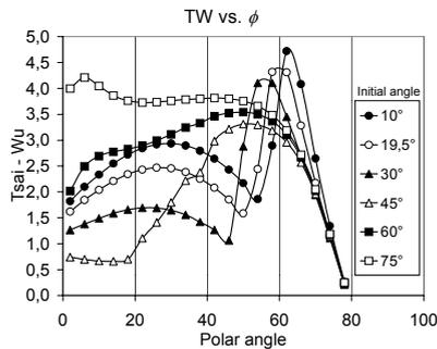
Figure 7: Influence of the initial winding angle on the sphere Tsai – Wu coefficient.
