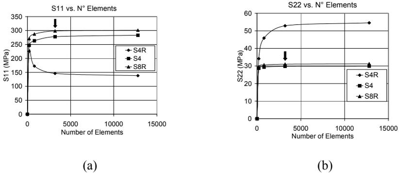
Figure 2: Comparison of the element types. (a) Stress 1 vs. Number of elements. (b) Stress 2 vs. Number of elements.
