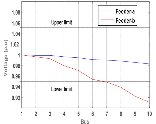
Figure 6. Voltage profile of the system buses in the case 1 without any controller.
