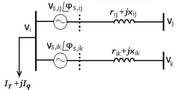
Figure 2. Equivalent circuit of GUPFC.
