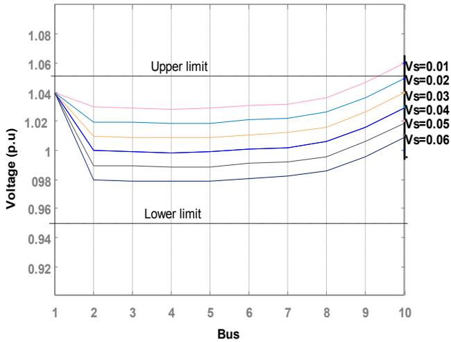
Figure 11. Voltage profile of the Feder-a in the case 2 with variation of  $V_s$ .
