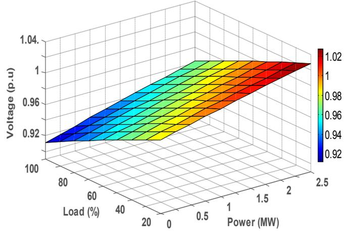
Figure 5. Voltage at bus 10 with variations of demand of the load and power of DG.
