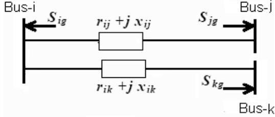
Figure 3. Injection model of GUPFC.
