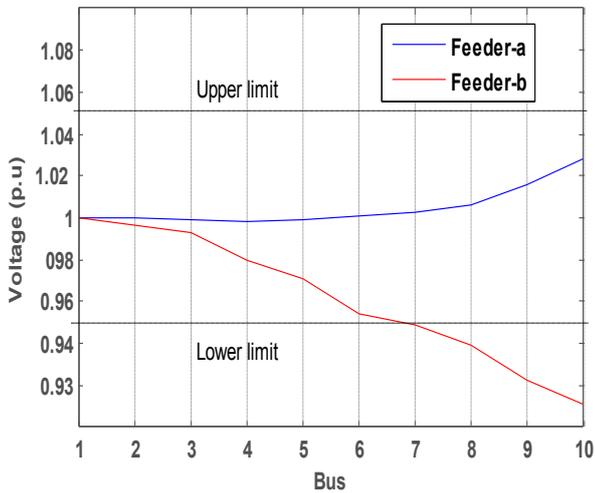
Figure 8. Voltage profile of the system buses in the case 2 without any controller.
