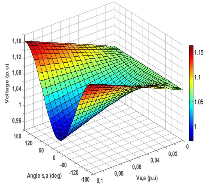
Figure 10. voltage at bus 10-a with the variation of magnitude and phase angle of serie injected voltage.
