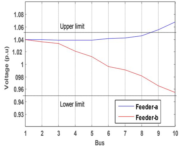
Figure 9. Voltage profile of the system buses in the case 2 with single action of OLTC.
