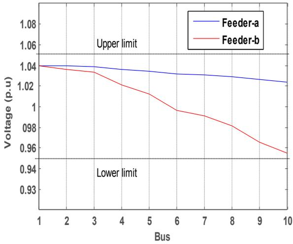
Figure 7. Voltage profile of the system buses in the case 1 with single action of OLTC.
