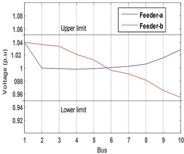
Figure 12. Voltage profile of the system buses in the case 2 with the proposed idea.
