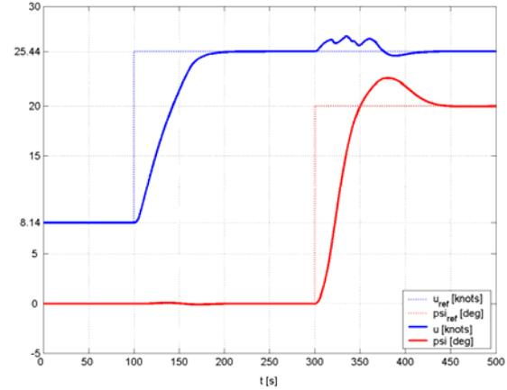
Figure 7. The course angle and speed of the ship.
