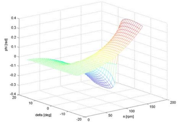
Figure 5. The roll angle in the nominal operating points.
