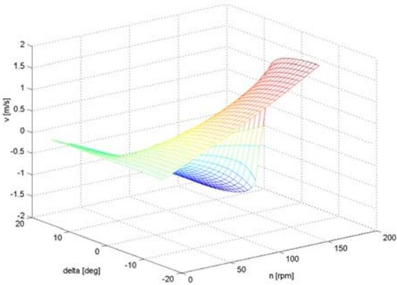
Figure 3. The sway velocity in the nominal operating points.
