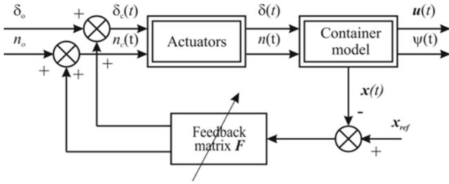
Figure 6. Block diagram of the proposed control system structure.
