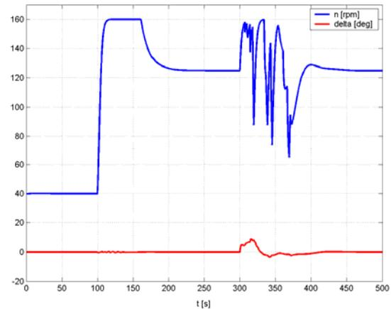
Figure 8. Rudder angle and shaft speed.
