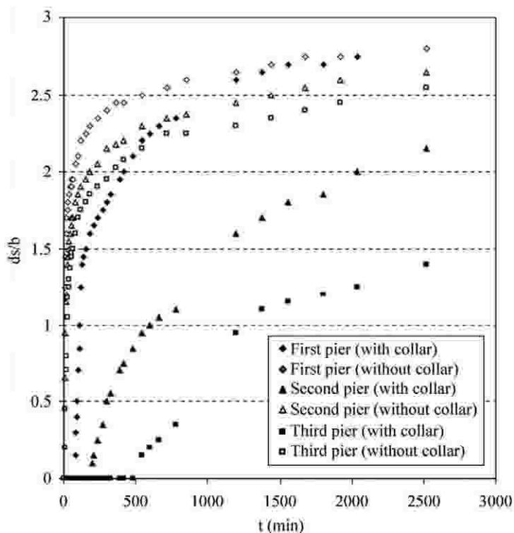
Fig. 7 Comparison of scouring depth at group of three piers with and without collar with  $S/b=3$  and  $w/b=3$
