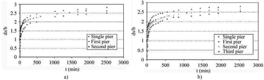
Fig. 5 Time development of scouring at a) single pier and group of two piers, b) single pier and group of three piers
