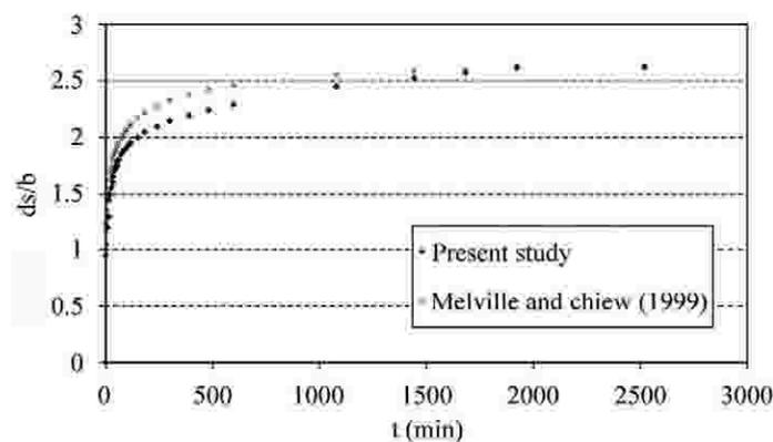
Fig. 4 Comparison of the experimental values of  $ds$  with the calculated ones by Melville and Chiew's equation
