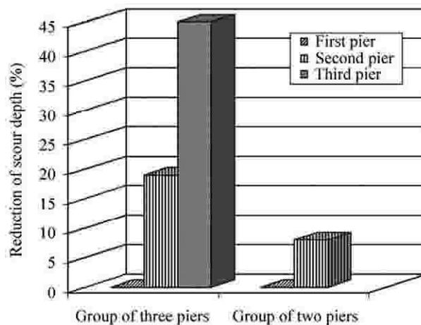
**Fig. 11** Reduction of scour depth at group of three and two piers with collar with  $S/b=3$ ,  $W/b=3$
