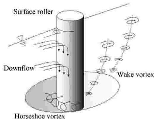
Fig. 1 Illustration of the flow and scour pattern at a circular pier
