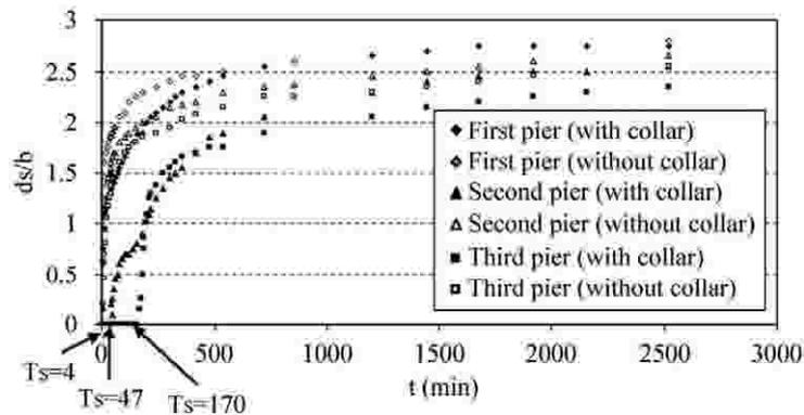
Fig. 8 Time development of scouring depth at group of three piers with and without collar with  $S/b=3$  and  $w/b=2$
