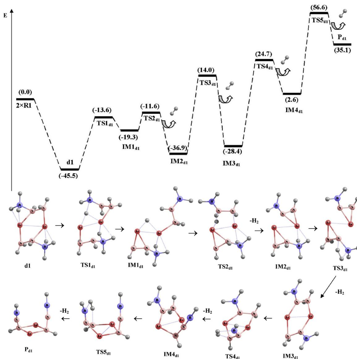
Fig. 6 – Dehydrogenation pathway of  $d1$  dimer, represented by both potential energy surface and schematic diagrams. Relative energies are in kcal/mol unit.
