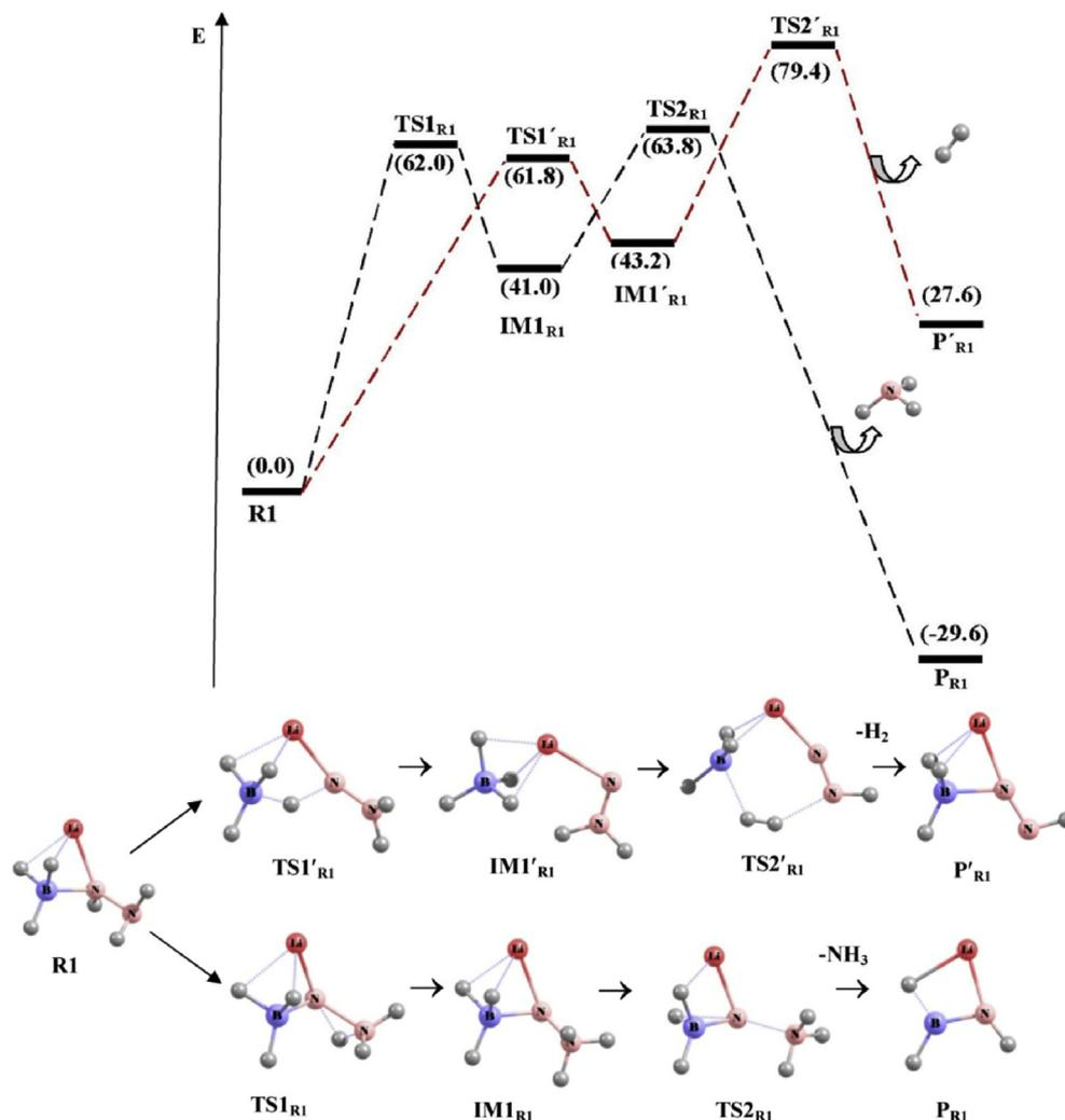
Fig. 2 – Decomposition channels of R1 isomer of  $\text{LiN}_2\text{H}_3\text{BH}_3$  represented by both potential energy surface and schematic diagrams. The pathway 1 and pathway 2 are denoted by black and red dashed lines respectively. Relative energies are in kcal/mol unit. (For interpretation of the references to colour in this figure legend, the reader is referred to the web version of this article.)
