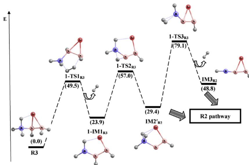
Fig. 5 – Decomposition channels of R3 isomer of  $LiN_2H_3BH_3$  (pathway 2), represented by both potential energy surface and schematic diagrams. Relative energies are in kcal/mol unit.
