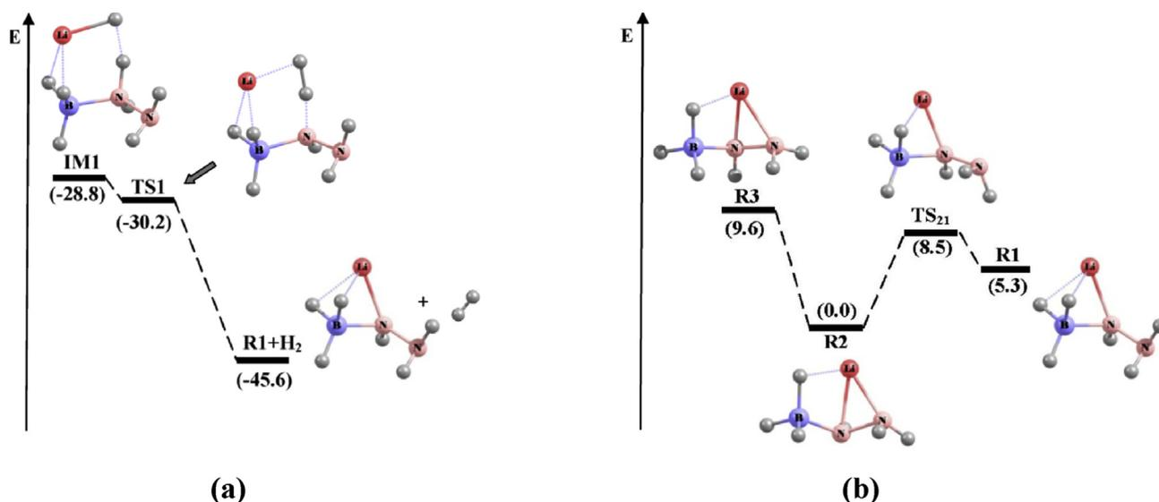
Fig. 1 – (a) Formation of LiN<sub>2</sub>H<sub>3</sub>BH<sub>3</sub> (R1) and (b) its subsequent isomerization. Relative energies are in kcal/mol unit.
