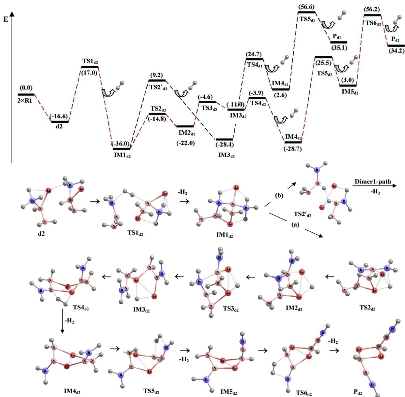
Fig. 7 – Dehydrogenation pathways of d2 dimer, represented by both potential energy surface and schematic diagrams. Relative energies are in kcal/mol unit.
