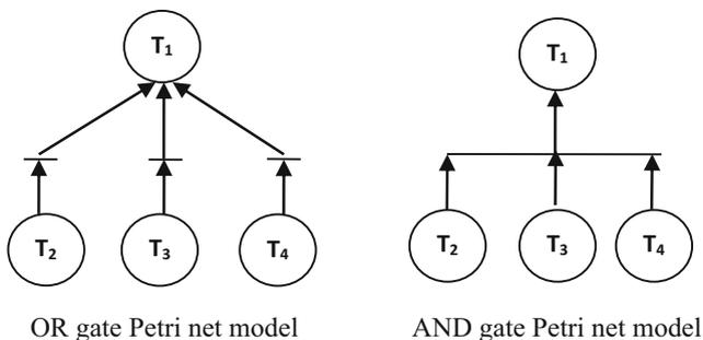
Fig. 2 PN model a OR gate b AND gate
