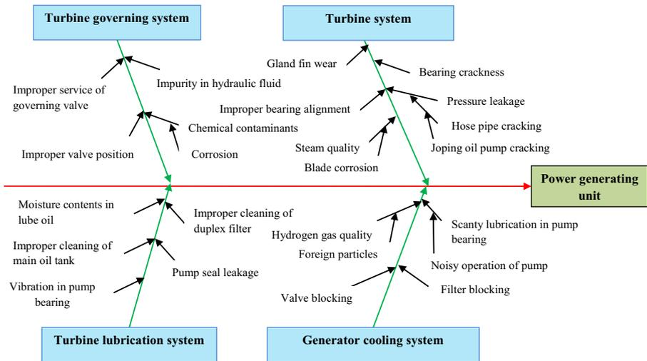
Fig. 11 Root cause analysis of PGU system
