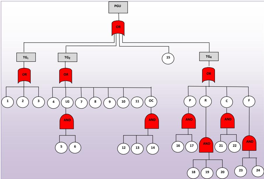
(a) Fault tree diagram for PGU
