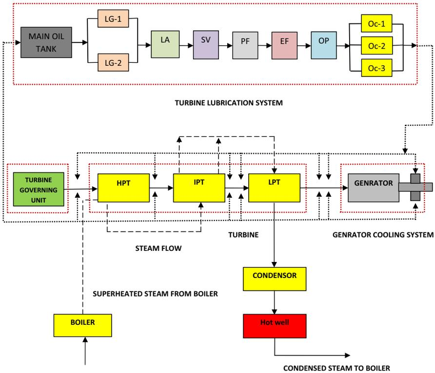
Fig. 5 Schematic diagram of PGU system
