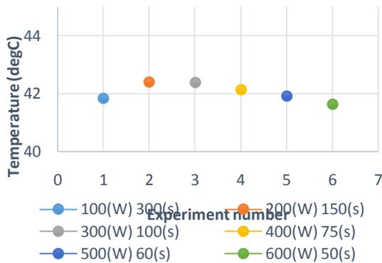
Figure 2. Temperature variations at fixed energy levels.
