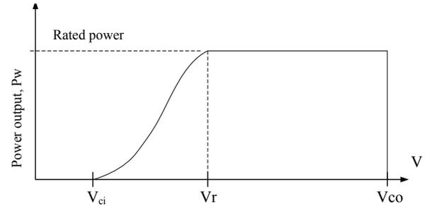
Fig. 2. Wind power output and wind speed relationship.
