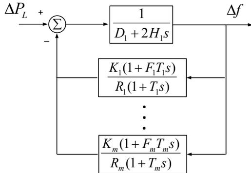
Fig. 4. Multi-machine LFC model [35].
