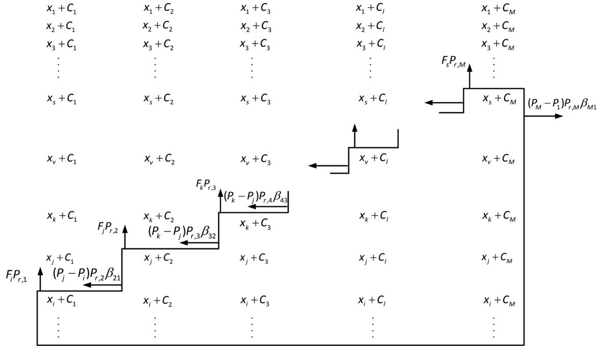
Fig. 6. State frequency diagram for unit addition.
