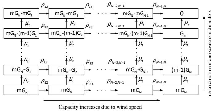
Fig. 3. State transition diagram for wind farm (the transitions between non-adjacent states are not shown for the sake of clarity).
