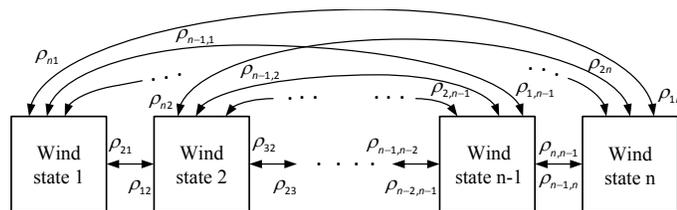
Fig. 1. Wind speed model with  $n$  states.
