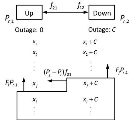
Fig. 5. Unit addition diagram for a two-state unit.
