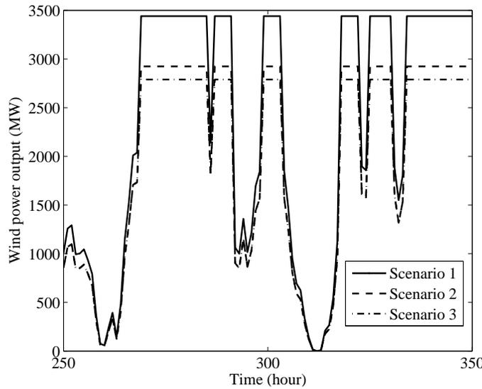
Fig. 7. Available wind output and integrated wind output for the scenarios.
