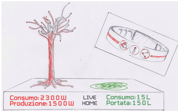
Fig. 1 One of the sketches related to the first project proposal, showing the main interface for the family and a sample of a complementary bracelet for the family's members. The base of the main artifact displays electricity production and consumption data ( on the left ) and water consumption data ( on the right )
