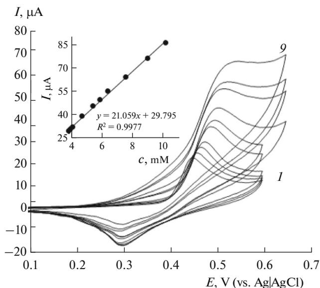
**Fig. 6.** Current–potential curves for oxidation of cabergoline at the Ni-NP/MCPE in 0.1 M NaOH solution with different concentrations of cabergoline: 0 (I), 0.005 (2), 0.05 (3), 0.5 (4), 0.8 (5), 0.1 (6), 1.5 (7), 2 (8) and 2.7 (9) mM. Inset: plot of  $I_p$  versus  $c$ .
