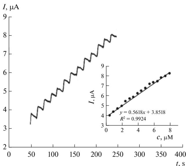
**Fig. 7.** Typical amperograms showing the current response for successive added volumes of 5  $\mu\text{M}$  solution of cabergoline in 0.1 M NaOH solution. Inset: variation of amperometric current vs. cabergoline concentration.
