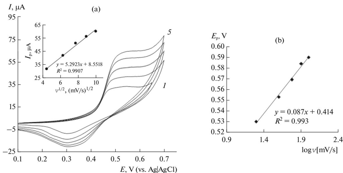
**Fig. 4.** (a)—Cyclic voltammograms of the Ni-NP/MCPE in 0.1 M NaOH solution containing 0.4 mM cabergoline at the scan rates, from 1 to 5: 20, 40, 60, 80, and 100 mV/s. Inset: variation of  $I_{pa}$  vs.  $v^{1/2}$ . (b)—Dependence of the peak potential,  $E_p$ , on  $\log v$  for the oxidation of cabergoline at Ni-NP/MCPE.
